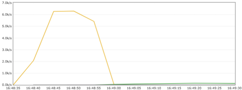
Figure 3-1. Snapshot of messaging rate to XML parser. The message rate is in yellow and message acknowledgement rate in green. With small message sizes RabbitMQ is able to scale up to thousands of messages per second before running out of data. Given a larger dataset one would expect message rates to continue increasing.
