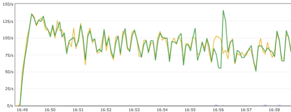
Figure 3-2. Snapshot of the message processing rate by the worker writing parquet data to the HDFS cluster. There is clearly a significant drop in processing rate compared to the messaging rate in Figure 3-1. The worker processes in this snapshot have significant latencies to deal with.
