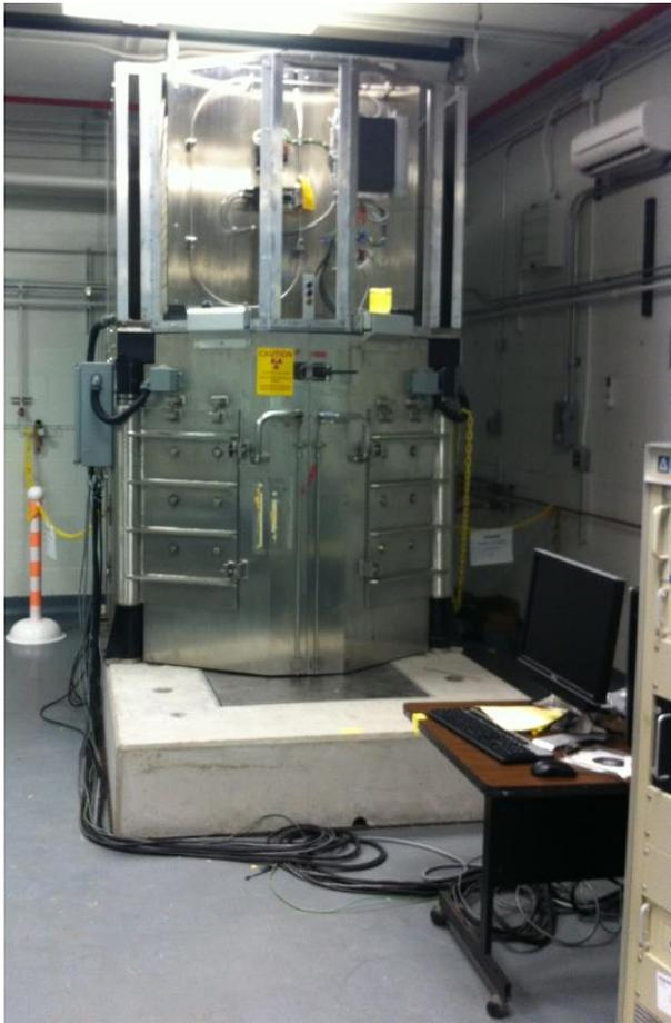
Figure 16. The  $^{252}\text{Cf}$  Shuffler at ORNL.
