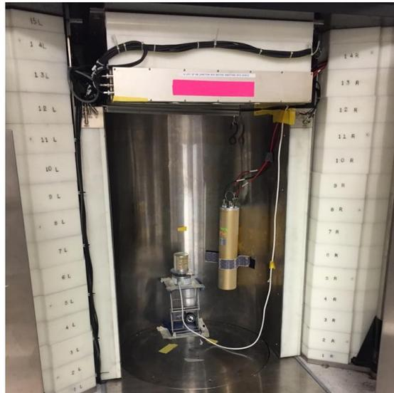
**Figure 36. Installed D-T generator.**
