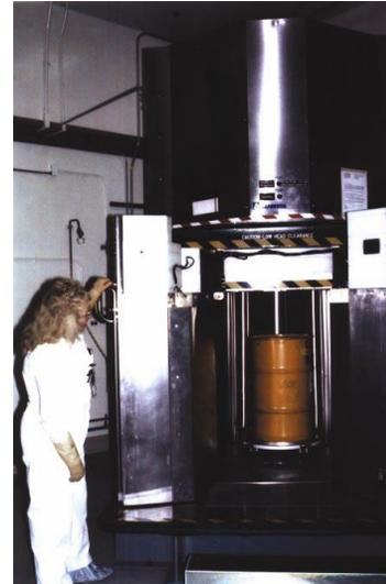
**Figure 12. Shuffler for 55 gal drums [29].**
