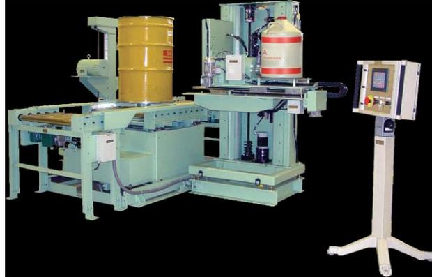
**Figure 14. Canberra TGS, which scans vertically and horizontally across the drum.**
