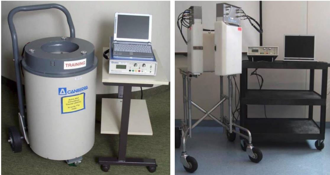
**Figure 6. AWCC and supporting electronics [14]. Figure 7. UNCL and supporting electronics [14].**
