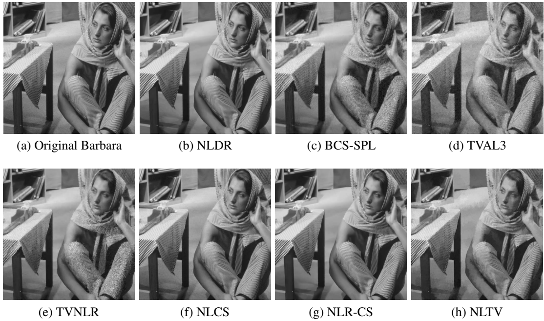
Figure 5.3: CS Reconstructed image Barbara with 30% measurement ratio. (a) Original image; (b) proposed NLDR recovery, PSNR=37.30dB; (c) BCS-SPL recovery Mun and Fowler (2009) , PSNR=25.92dB; (d) TVAL3 recovery Li et al. (2009a) , PSNR=24.79dB; (e) TVNLR recovery Zhang et al. (2013) , PSNR=25.35dB. (f) NLCS recovery Shu et al. (2014) , PSNR=31.65dB; (g) NLR-CS recovery Dong et al. (2014a) , PSNR=34.26dB; (h) NLTV recovery Zhang et al. (2010) , PSNR=31.79dB.
