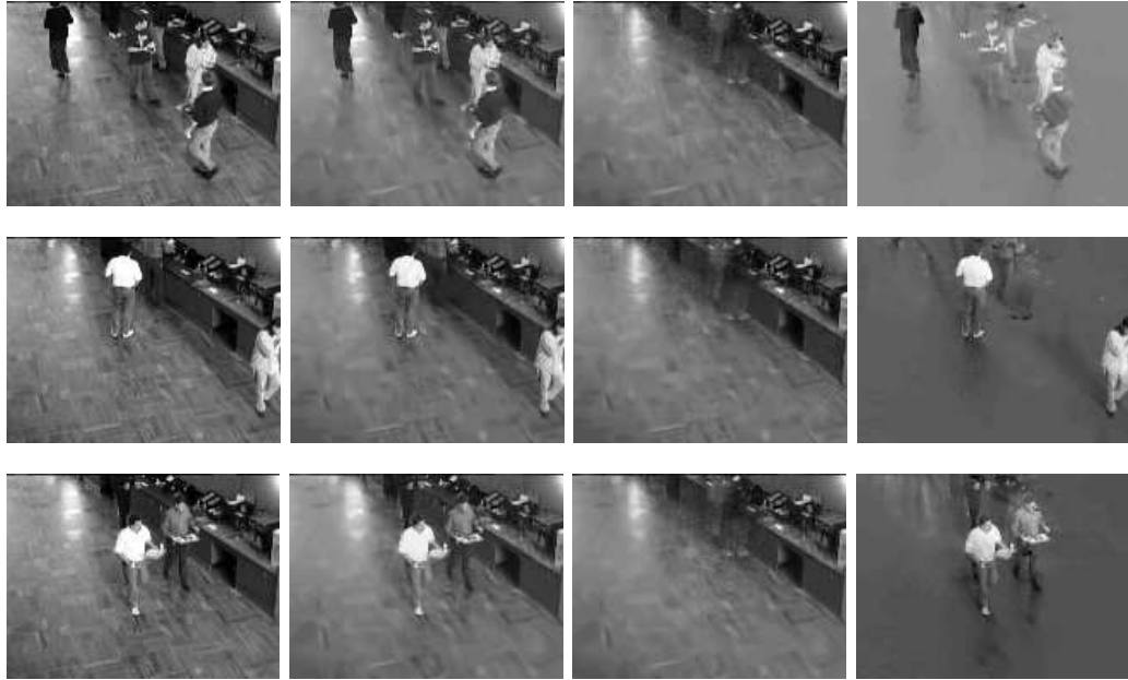
Figure 6.2: First column: original Restaurant video frames at t = 70, 116, 140 . Second column: frame recovered by NLDR with 30% measurements. Next 2 columns: background and object estimated by rLSDR .
