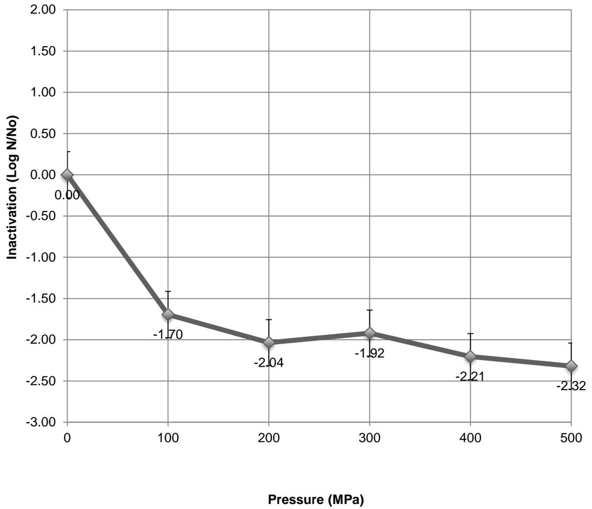
Figure 2.10. Inactivation of *Paenibacillus lautus* spores in apple juice using ultra-high pressure homogenization and no post treatment heat shock.
