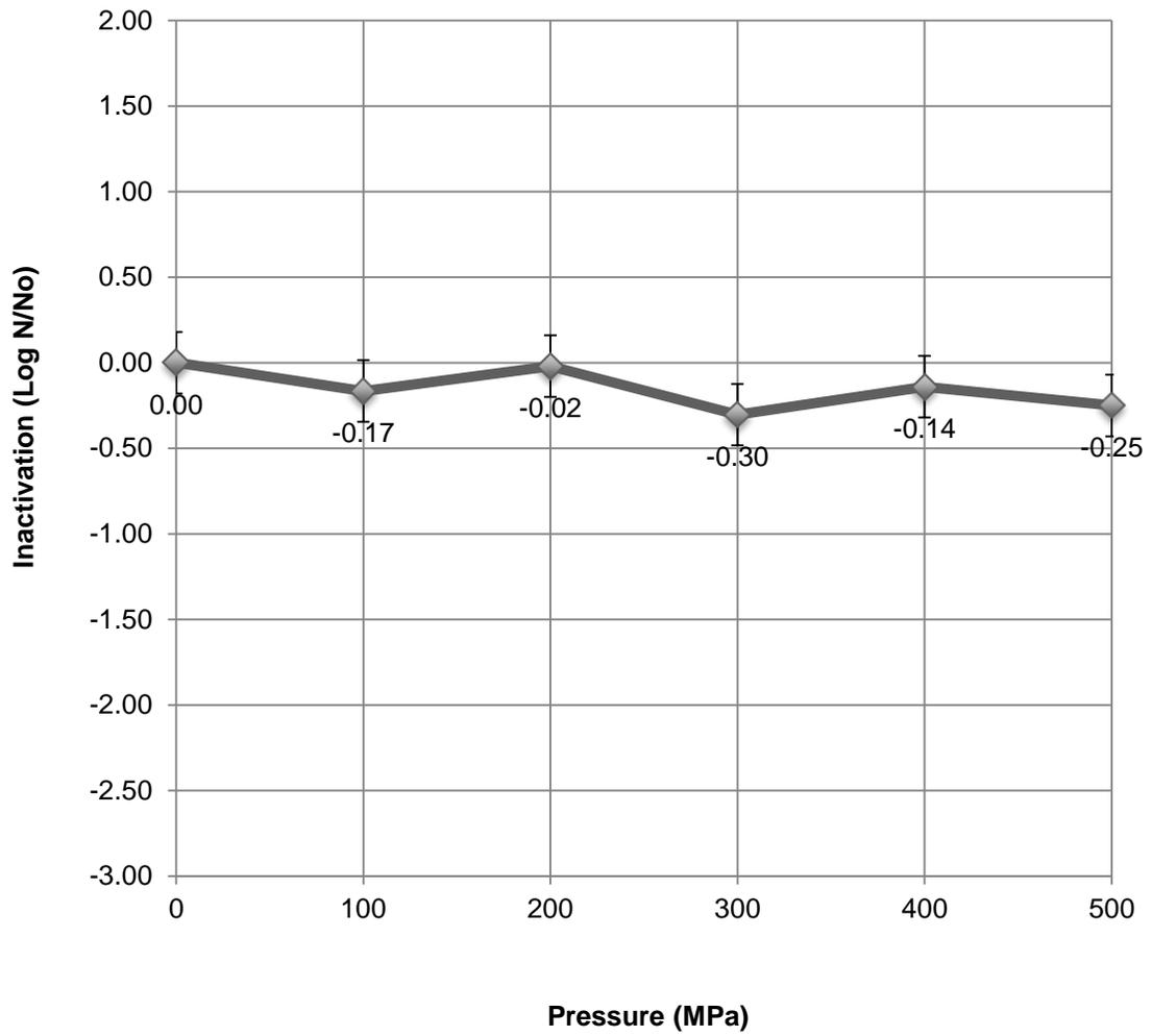
Figure 2.5. Inactivation of *Bacillus licheniformis* spores by ultra-high pressure homogenization with heat shock at 80°C for 10 min.
