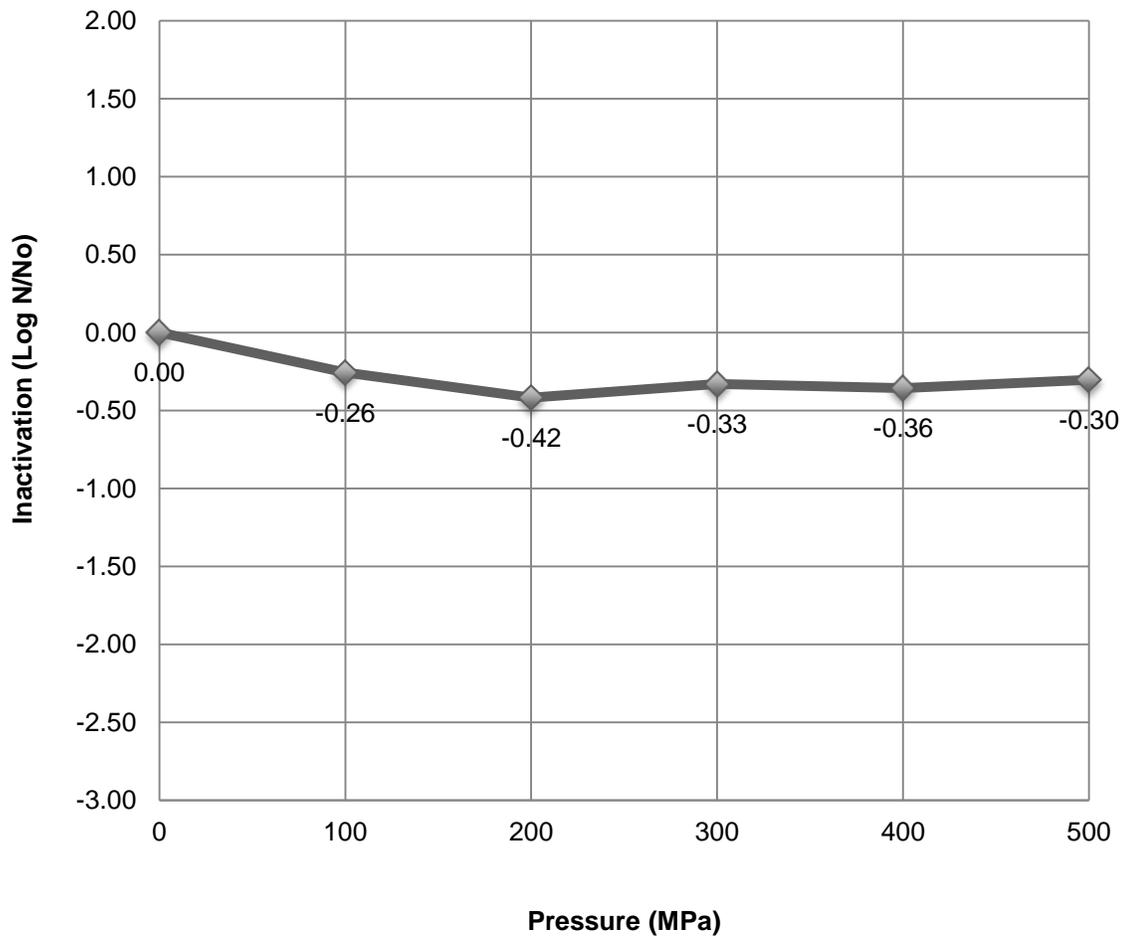
Figure 2.7. Inactivation of *Paenibacillus lautus* spores in non-fat organic milk using ultra-high pressure homogenization at 95°C and a post treatment heat shock at 80°C for 10 min.
