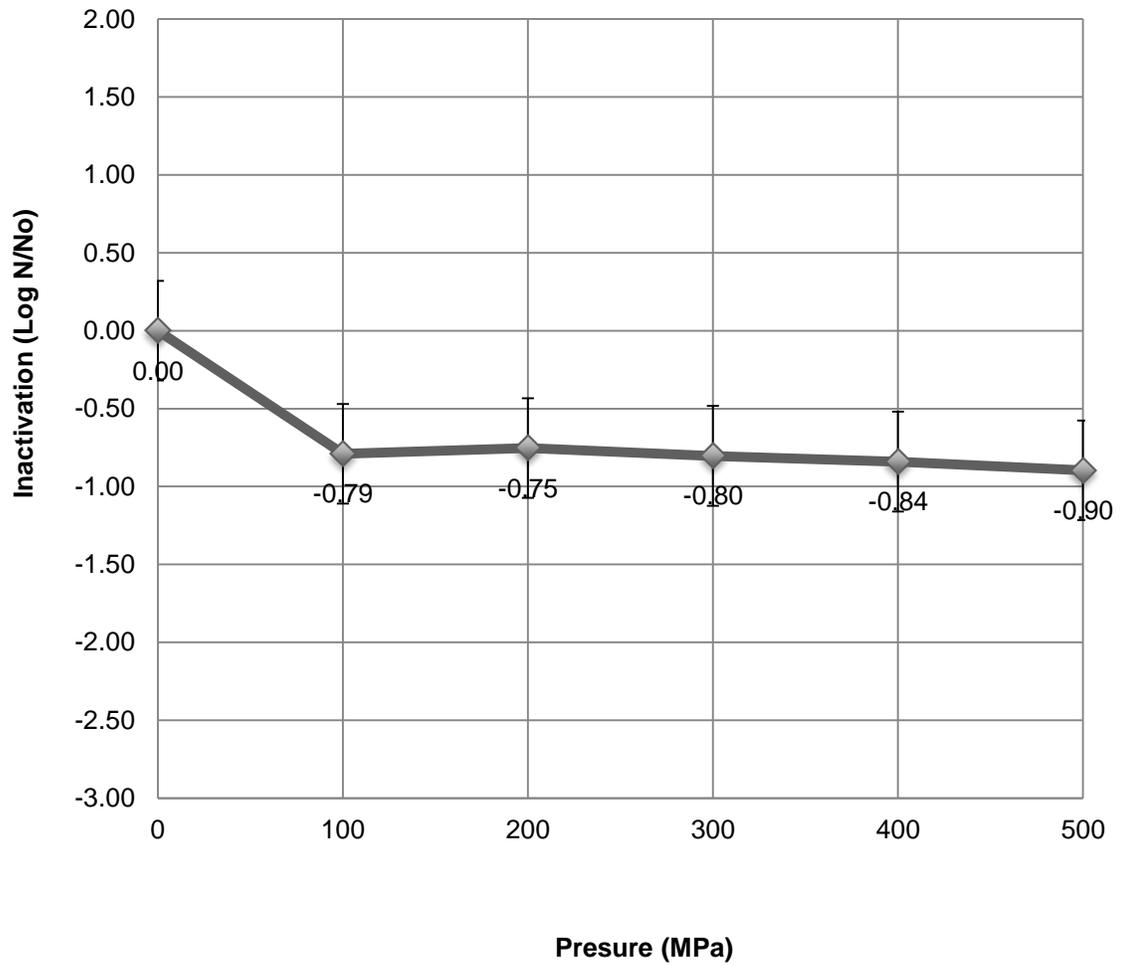
Figure 2.8. Inactivation of *Paenibacillus lautus* spores in non-fat organic milk using ultra-high pressure homogenization at 95°C and no post treatment heat shock.
