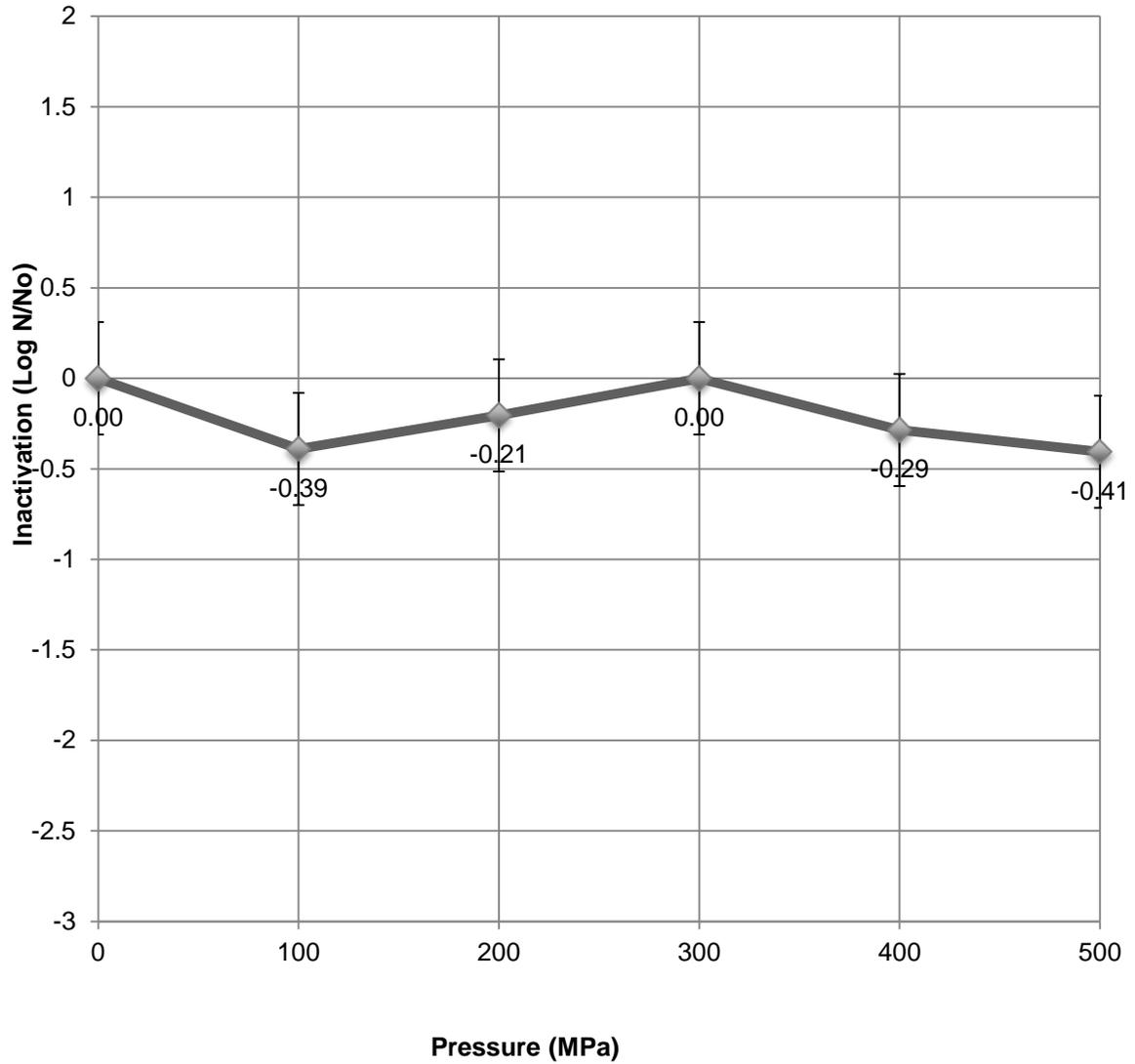
Figure 2.1. Inactivation of *Geobacillus stearothermophilus* spores by ultra-high pressure homogenization with heat shock at 80°C for 10 min.
