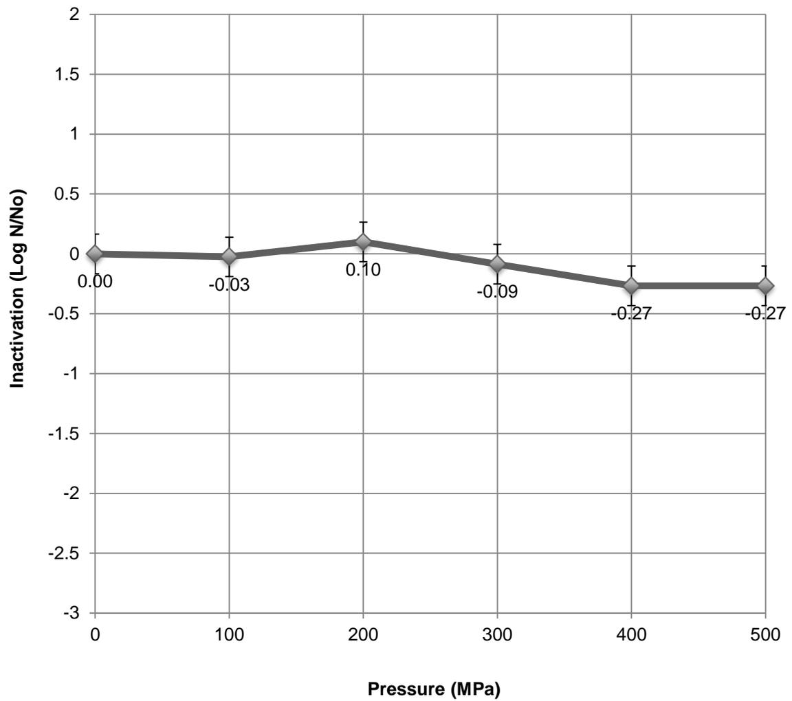
Figure 2.6. Inactivation of *Bacillus licheniformis* spores by ultra-high pressure homogenization without heat shock.
