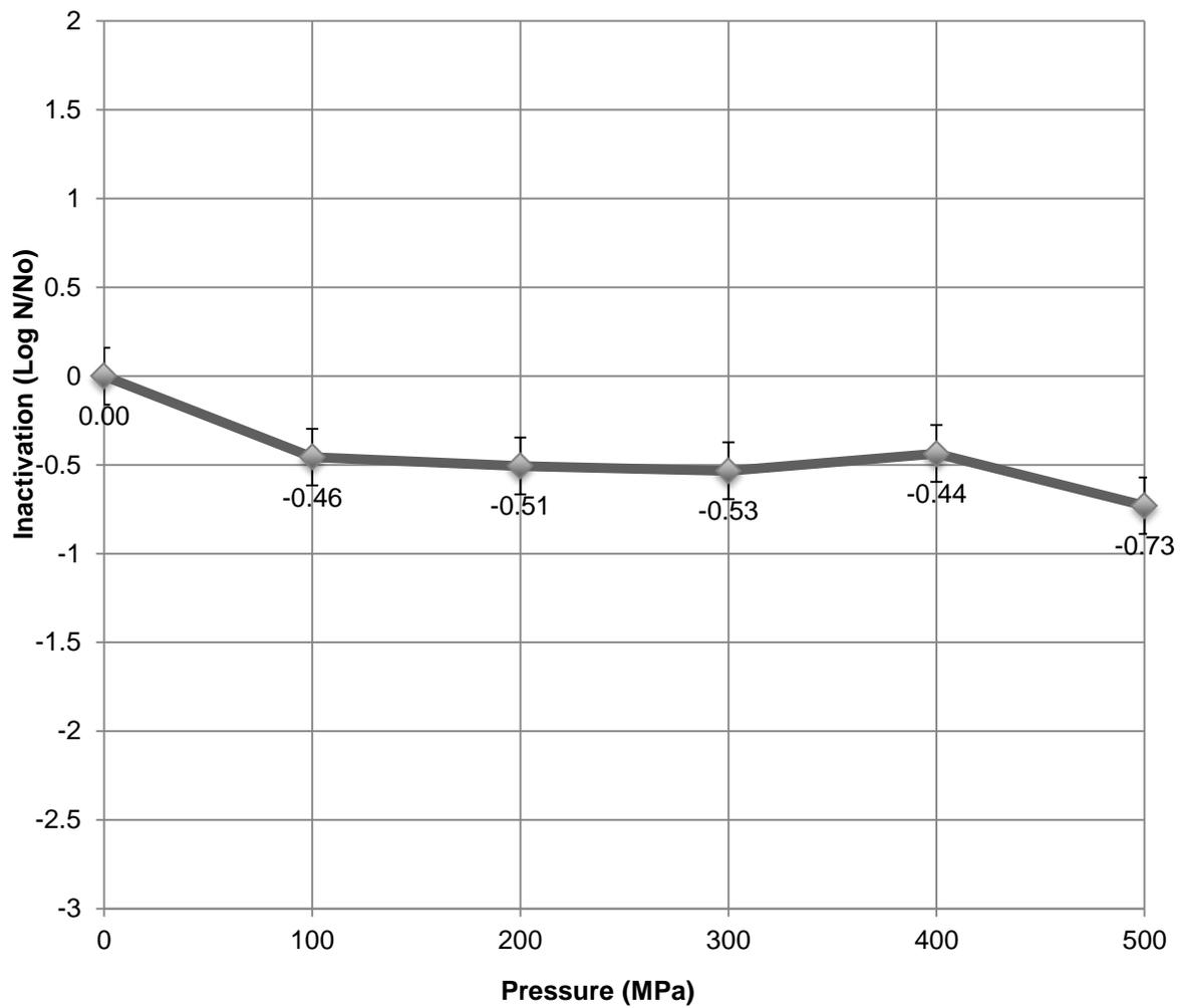
Figure 2.3. Inactivation of *Paenibacillus lautus* spores by ultra-high pressure homogenization with heat shock at 80°C for 10 min.
