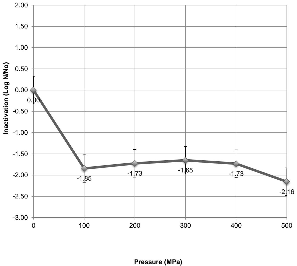
Figure 2.9. Inactivation of *Paenibacillus lautus* spores in apple juice using ultra-high pressure homogenization and a post treatment heat shock at 80°C for 10 min.
