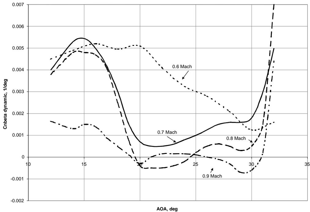
**Figure 12 - Departure resistance of the single seat aircraft with the centerline tank, at various Mach numbers**
