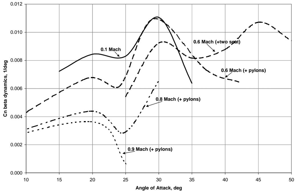
**Figure 15 – Departure resistance with two wing fuel tanks**
