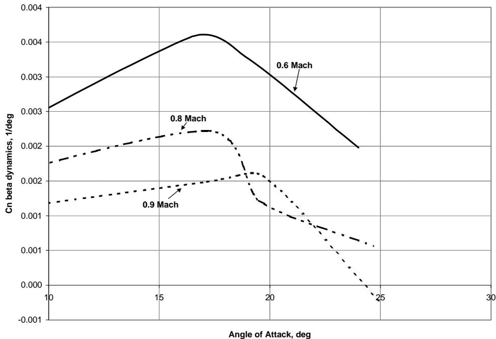
**Figure 16 – Departure resistance of the single seat aircraft with Interdiction loading**
