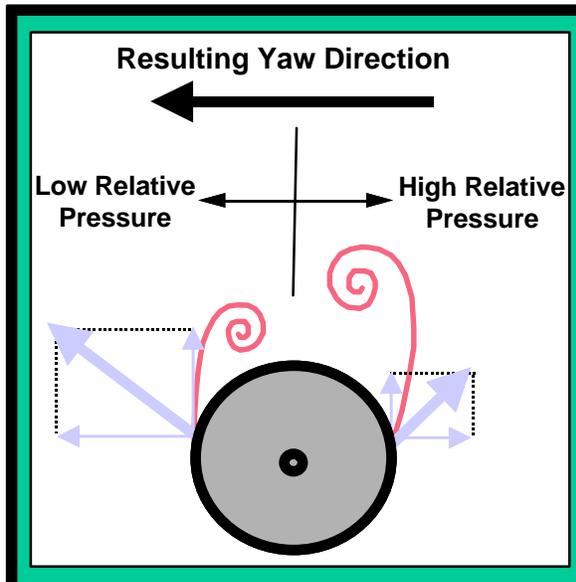
**Figure 7 – Force Generated by Asymmetric Vortex Separation**
