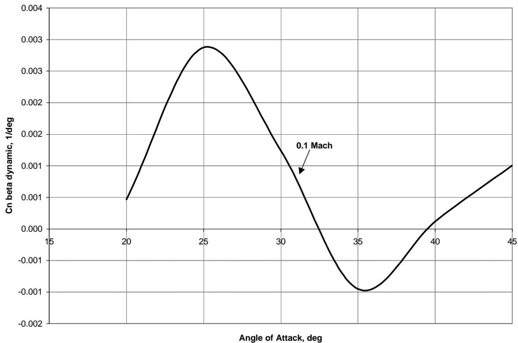
**Figure 14 – Departure resistance of the two seat aircraft with asymmetric wingtip missile loaded (left wingtip)**
