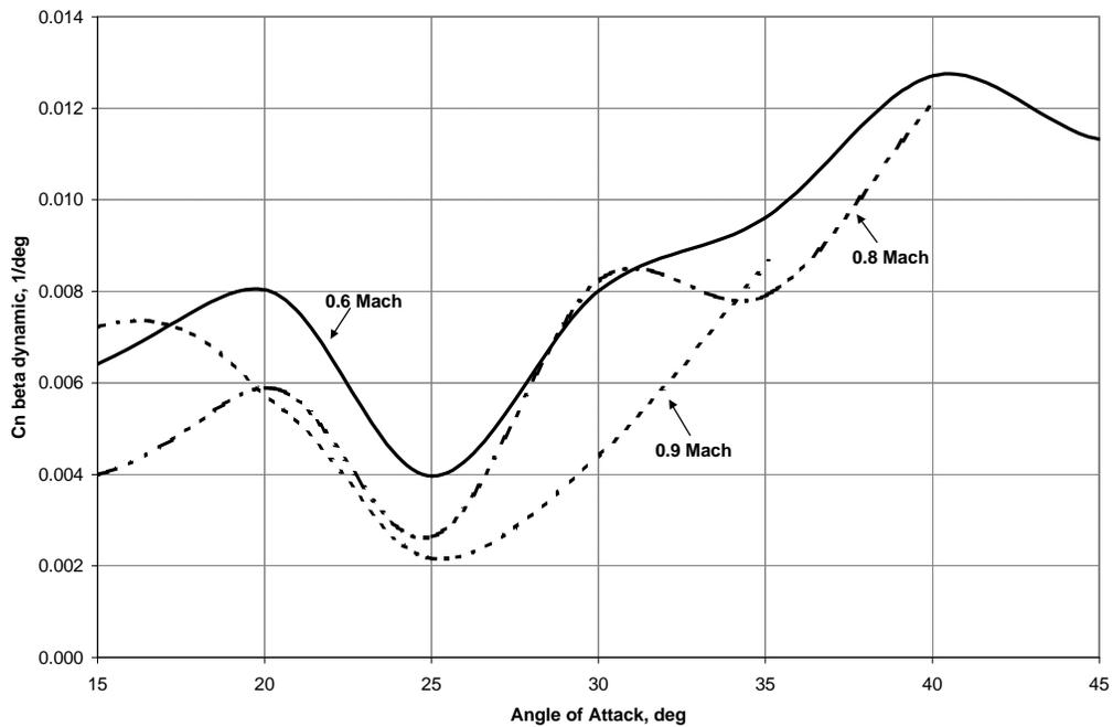
**Figure 19 – Departure resistance of the two seat aircraft with the RECCE nose**
