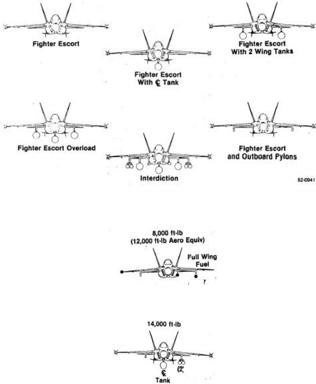
Figure A1 - F/A-18A/B/C/D Configuration Examples
