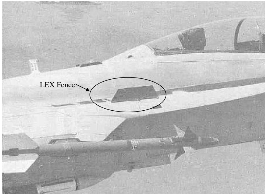
**Figure 3 – Leading edge extension fence modification (ref 15)**
