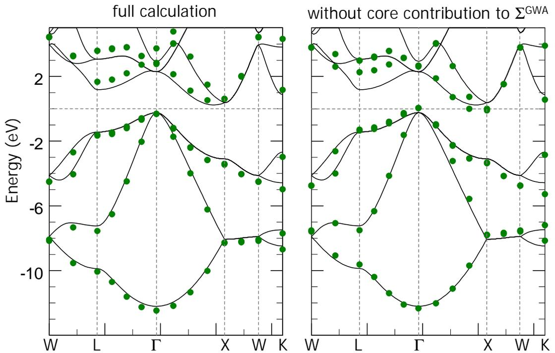
Figure 13 Significance of Core Contribution: QP band structure of Si
