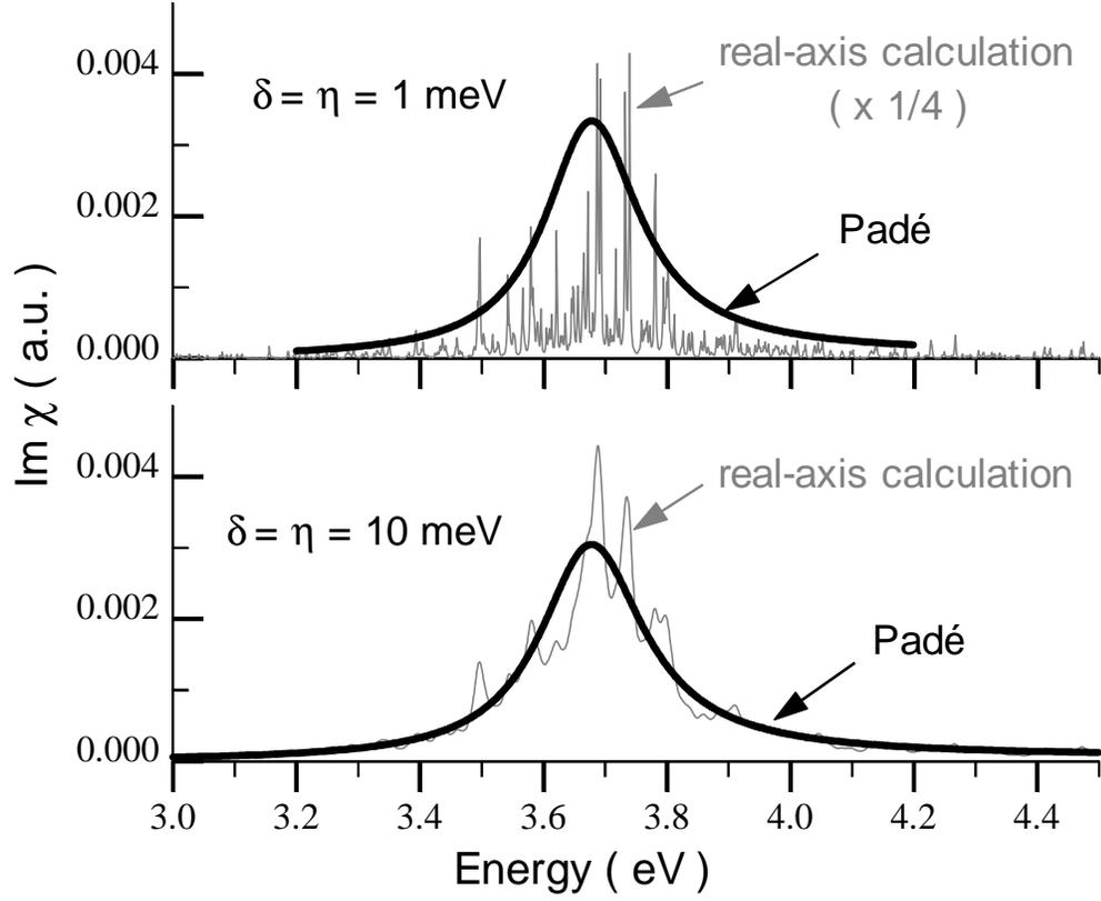
Figure 1 Imaginary Sampling Technique : loss function for K
