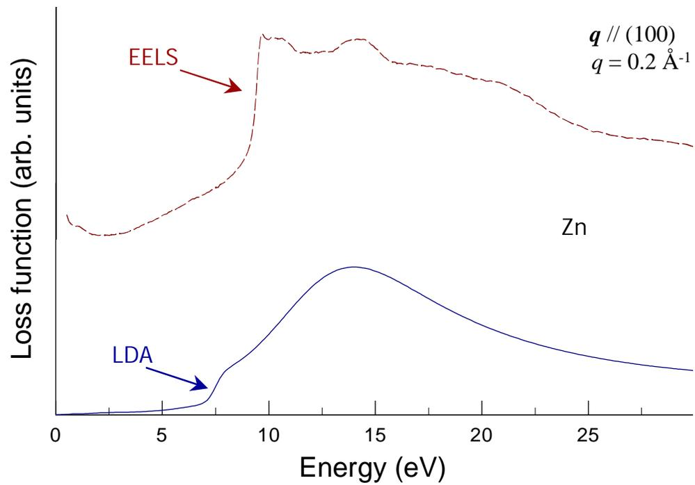
Figure 6 Failure of the LDA Based Dynamical Response: loss function of Zn
