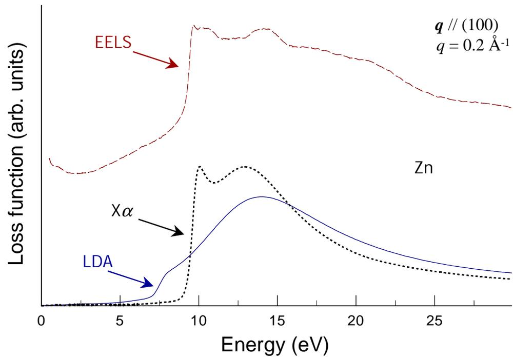
Figure 9 Phenomenological Simulation of Dynamical Response in Zn
