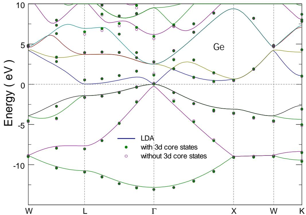
Figure 15 Impact of Core Polarization: QP band structure of Ge
