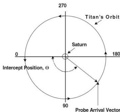
**Figure 1: Coordinate system used for Titan arrival geometry.**
