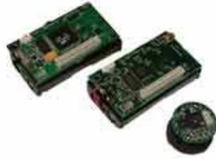
Figure 1.2: The Motes from Crossbow Corporation. Left: MICA; Middle: MICA2; Right: MICA2DOT [46].
