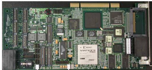
Figure 4.63: The Amirix platform embedded with Xilinx Virtex II Pro FPGA.
