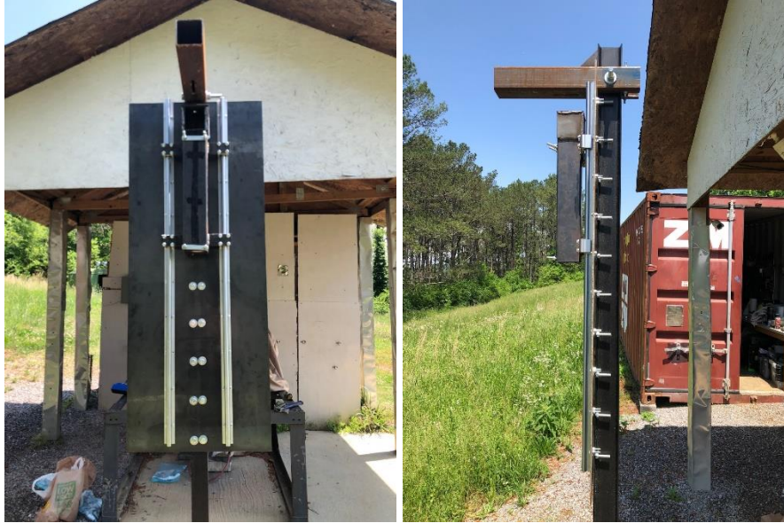
Fig. 7 This figure shows the completed vertical test stand.
