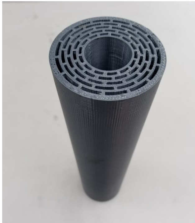
Fig. 1 Polymer matrix fuel grain. The one-inch diameter, single combustion port is in the center. Powdered, non-melting fuel is placed in the void spaces.
