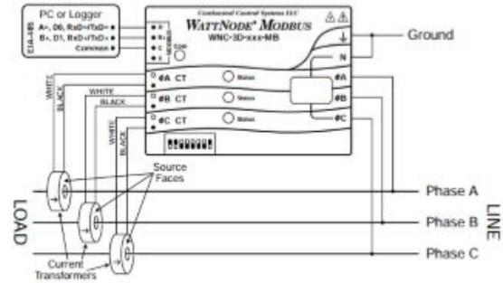
Take care to orient the CTs facing the source of power. Labels on CTs indicate direction. Be sure to keep track of conductor phase for each CT.
