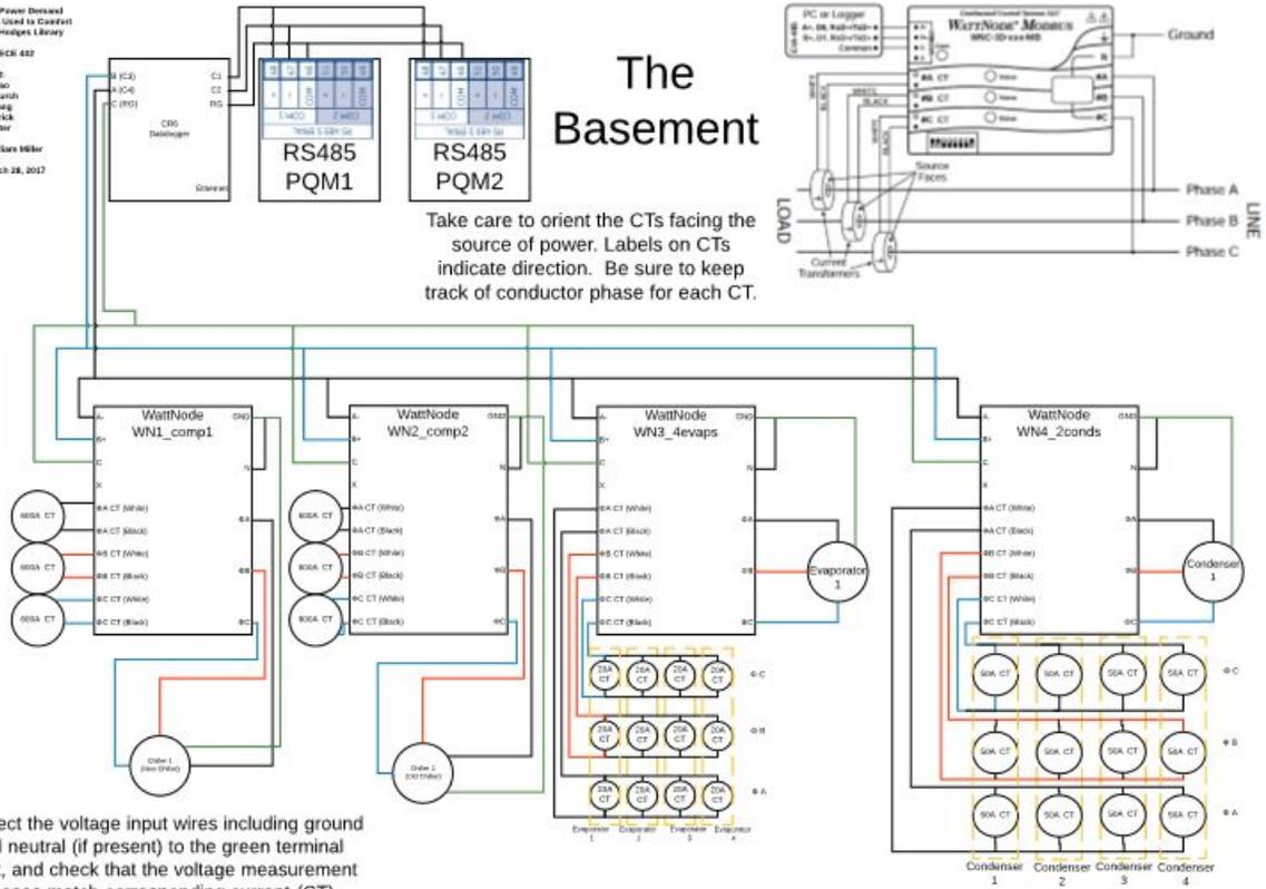
Connect the voltage input wires including ground and neutral (if present) to the green terminal block, and check that the voltage measurement phases match corresponding current (CT) phases. If neutral is not present, then short the wattnode's N terminal to ground as shown. Use 14 AWG stranded conductors rated for > 480VAC.
