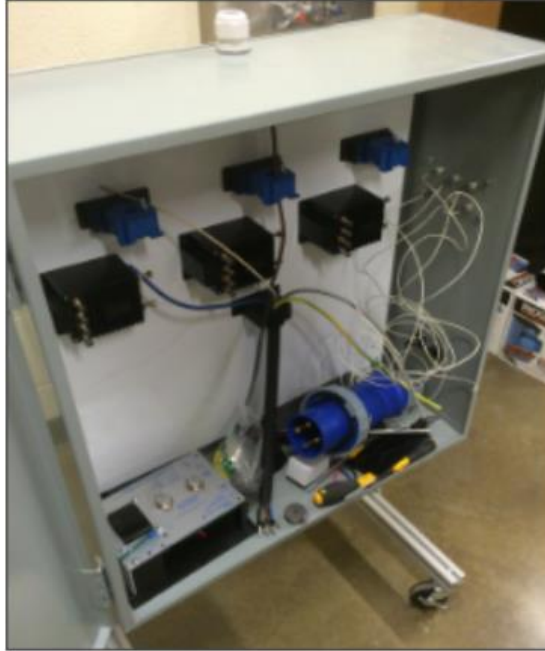
Figure 2.10a: Original AMPCMS Design, Internal Components
