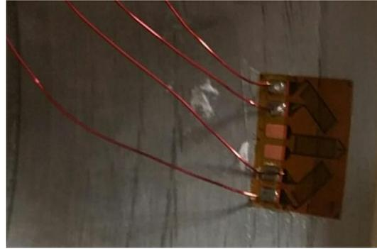
*Figure 8: Mounted Strain Gauge*
