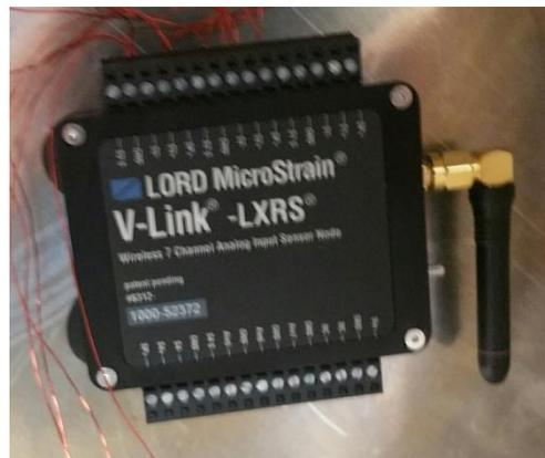
*Figure 9: Wireless Node by LORD MicroStrain*
