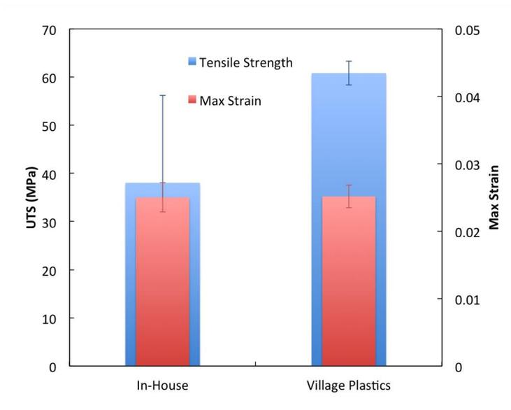
**Figure 5.** Average tensile strength and max strain of in-house extruded filament compared to Village Plastics filament. Error bars show one standard deviation of error.
