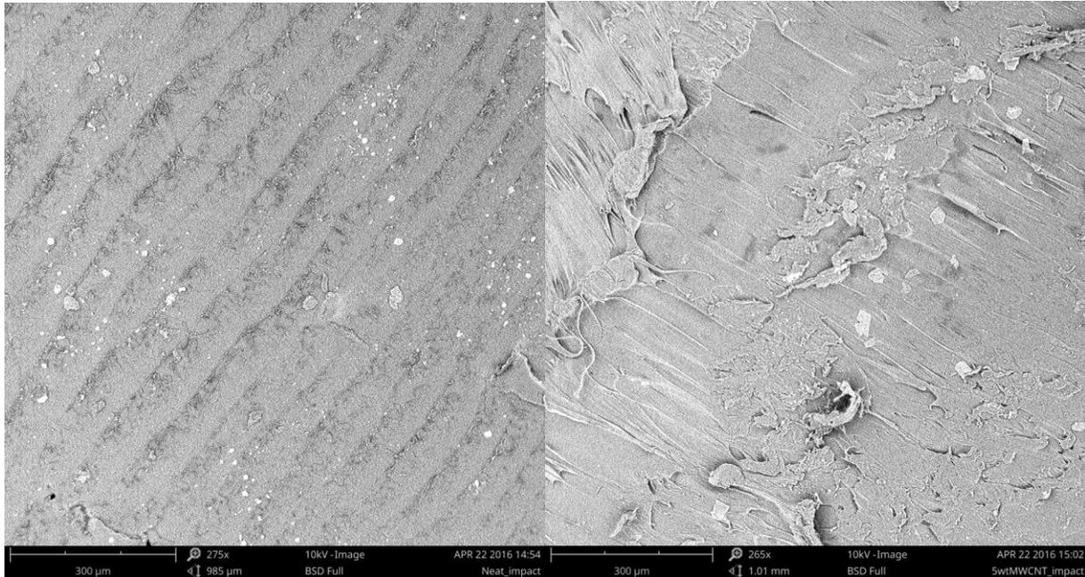
**Figure 9.** Fracture surface of a neat printed PLA bar (left) and 5 weight percent carbon nanotube printed bar (right).
