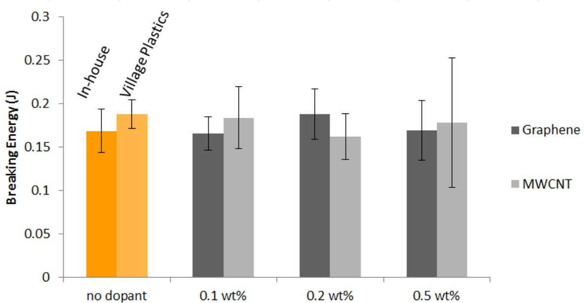
**Figure 8.** Impact testing results for graphene and carbon nanotube composites and neat in-house and Village Plastics PLA.
