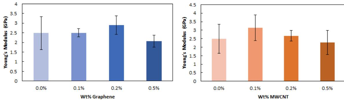
**Figure 3.** Average Young's Modulus of each composition tested. Error bars show one standard deviation of error.
