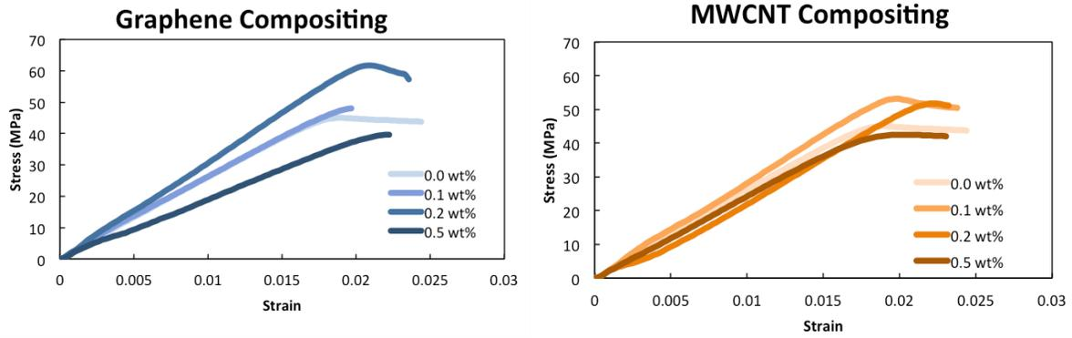
**Figure 1.** Representative stress-strain curves for all compositions tested
