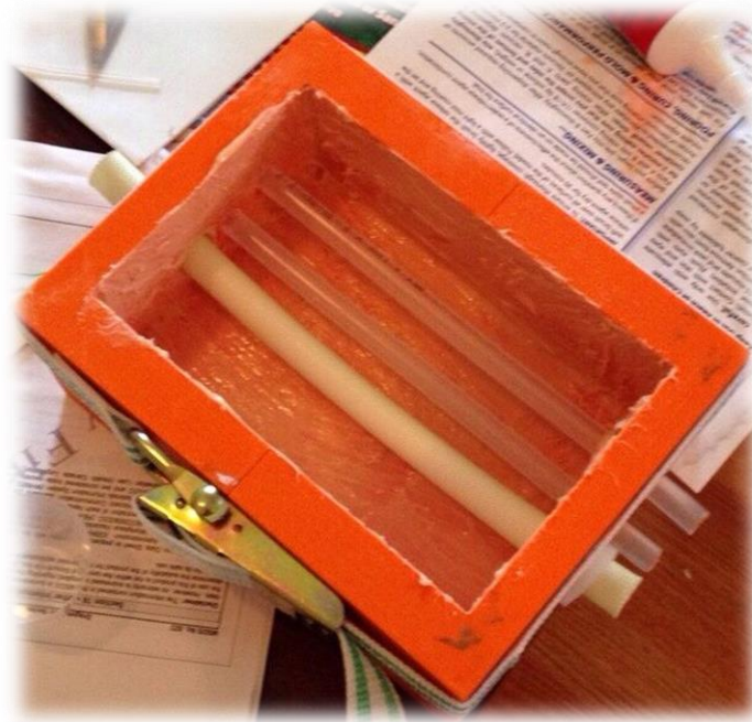
Figure 3: Shows the inside of the mold coated with Dragonskin and Thivex and the internal structures that been added to the mold by being held in the holes in the sides of the mold.
