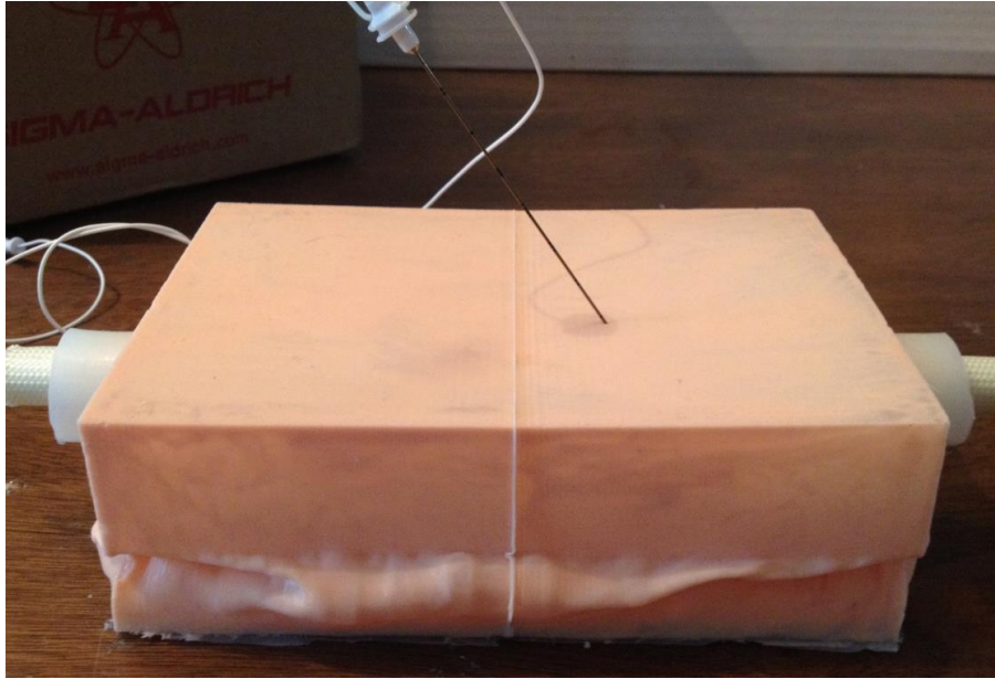
Figure 6: The first model that did not create a satisfactory ultrasound and had a large air pocket inside due to the size of the lung.
