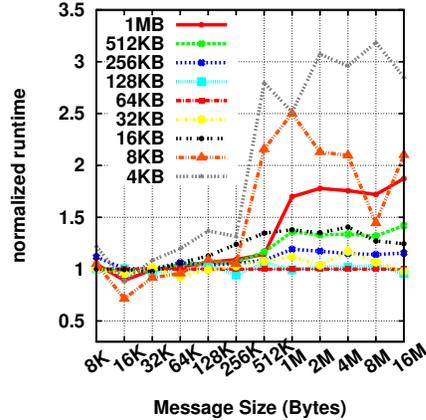
**Figure 5.2:** Effect of Pipeline Size on HierKNEM Broadcast Execution Time (Paraplume cluster: 768 Processes, 32 compute nodes, InfiniBand 20G); Runtime is normalized to the result for 64KB pipeline size (the smaller, the better).
