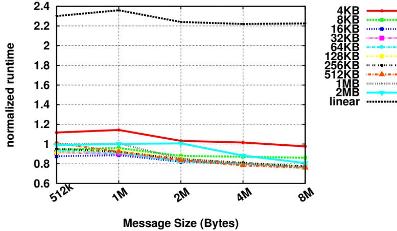
**Figure 3.6:** Performance comparison between linear KNEM Broadcast, hierarchical KNEM without pipeline, and different pipeline sizes in the hierarchical pipelined KNEM Broadcast on the IG platform. Results are normalized to the runtime of hierarchical KNEM Broadcast without pipeline (lower is better).
