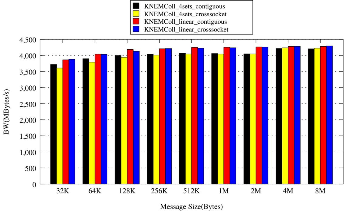
**Figure 4.8:** Bandwidth Comparison of KNEM Broadcast on Zoot with 16 processes over two different topologies: 4 sets and linear, between 2 binding cases: the contiguous case and the cross socket case.
