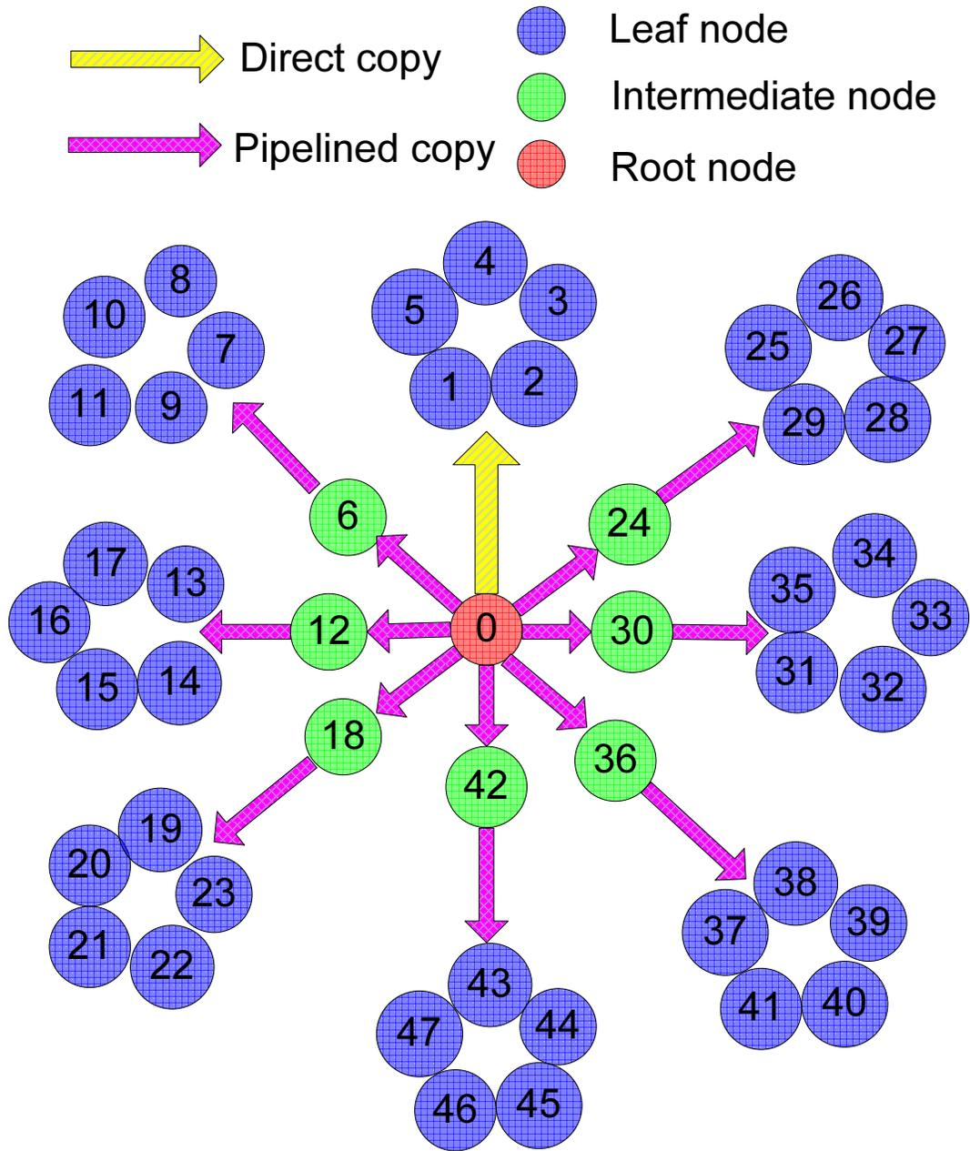
**Figure 3.3:** Progression of the hierarchical pipeline KMEM Broadcast
