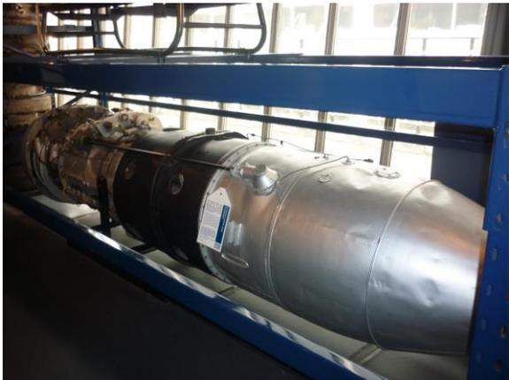
Junkers Jumo 004B turbojet, first-ever to see service and typical powerplant for Messerschmitt Me 262
