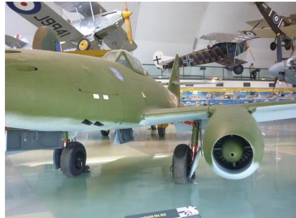
Messerschmitt Me 262, first operational jet fighter, powered by either Jumo 004 or BMW 003 engines
