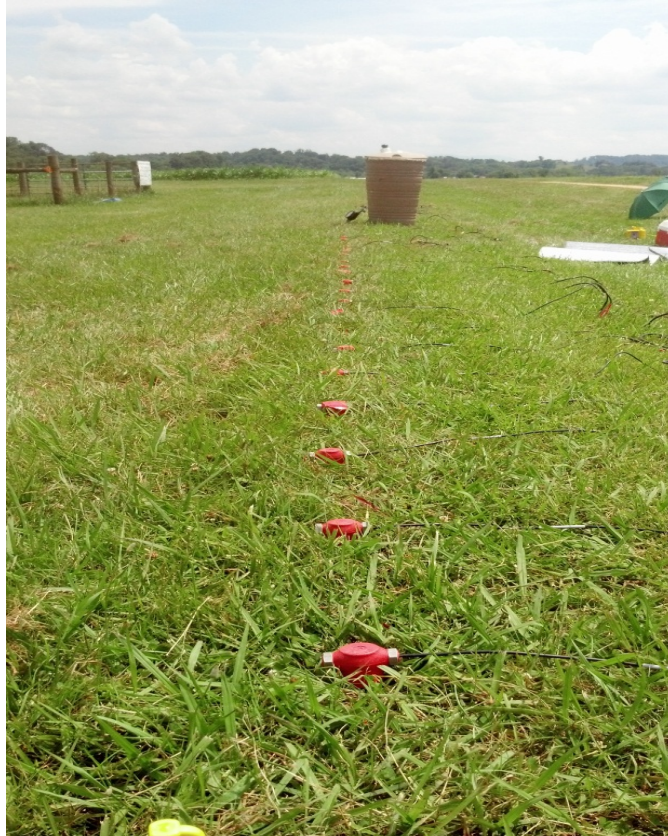
Figure 5: Field image of profile transect with seismic equipment employed. The red geophones can be seen in the foreground and the green plastic barrel is located in the middle of the profile transect.
