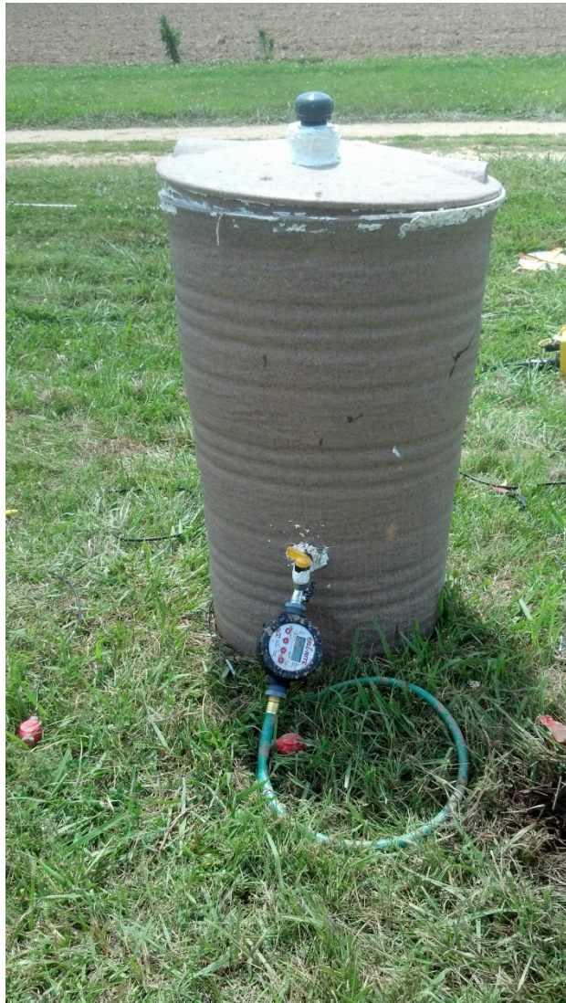
Figure 29: Photograph of the second constant flux applicator apparatus used for the infiltration experiment. The plastic barrel was centered along the profile transect, and the hose was used to infiltrate water into augured well.
