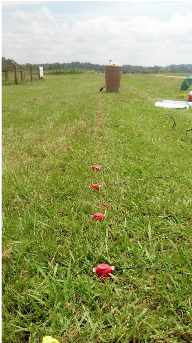
Figure 28: Photograph of the profile transect at the B-4 plot with seismic equipment employed for the second constant flux applicator infiltration experiment. The red geophones can be seen in the foreground and the green plastic barrel is located in the middle of the profile transect.
