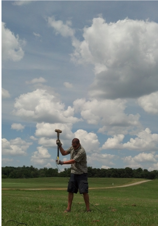
Figure 7: Image displaying the seismic source used for each seismic profile collected. At each shot point within the seismic profiles, a sledge hammer and metal strike-plate were used to generate a manual seismic source.
