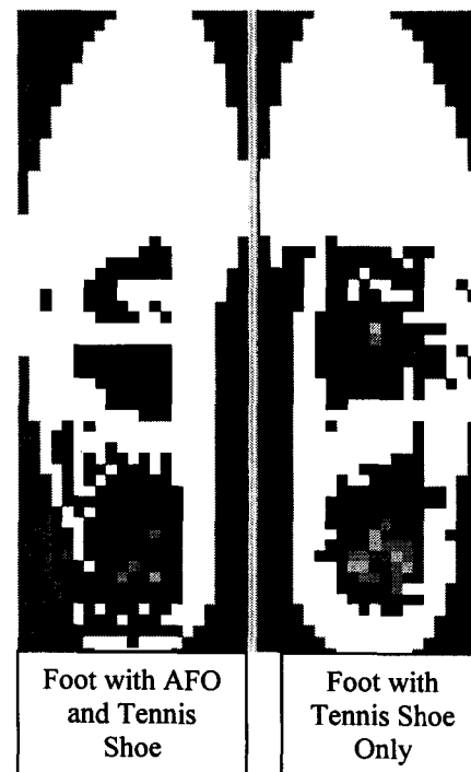
Figure 12. Pressure on foot when patient is wearing the AFO and the tennis shoe versus wearing the tennis shoe only. The foot with the AFO has no points of very high
