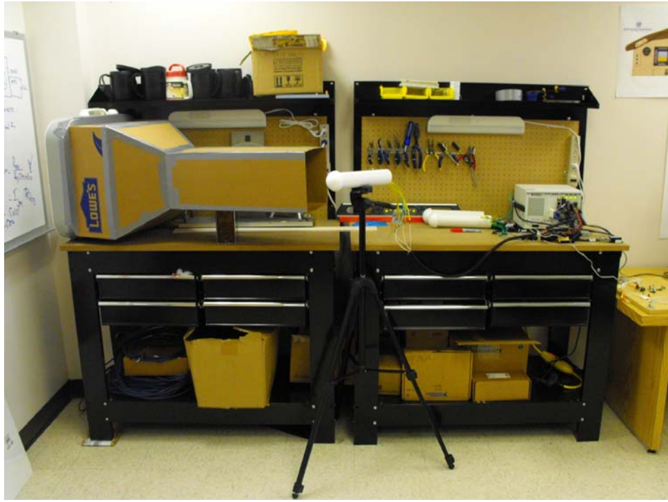
Figure 7. Bench test set up, showing probe head, wind generator and PXI device.
