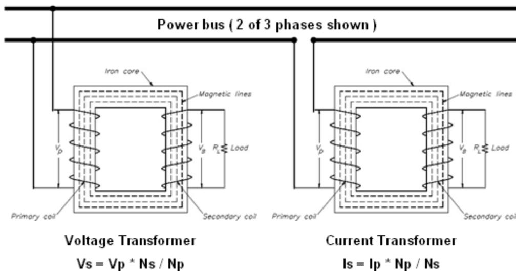
**Figure 3.1. Illustration of existing instrument transducer technology**
