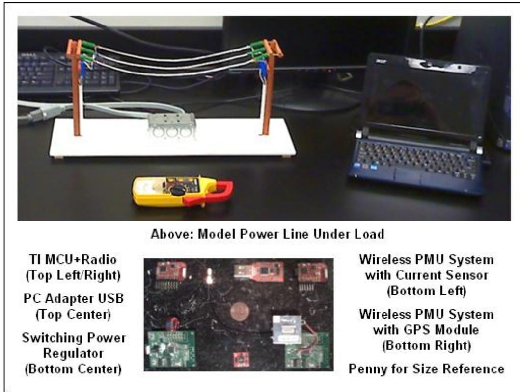
***Figure 4.3. Author's hardware prototype and model power line***
