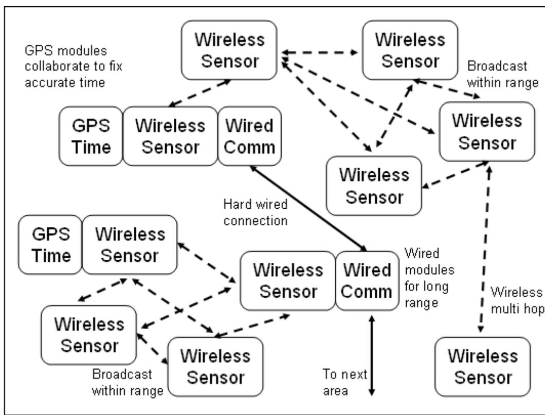
**Figure 3.2. High level system timing view [18]**
