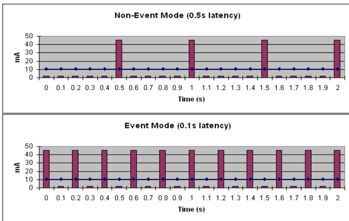
**Figure 4.10. Power harvesting (lines) versus power consumption (bars)**
