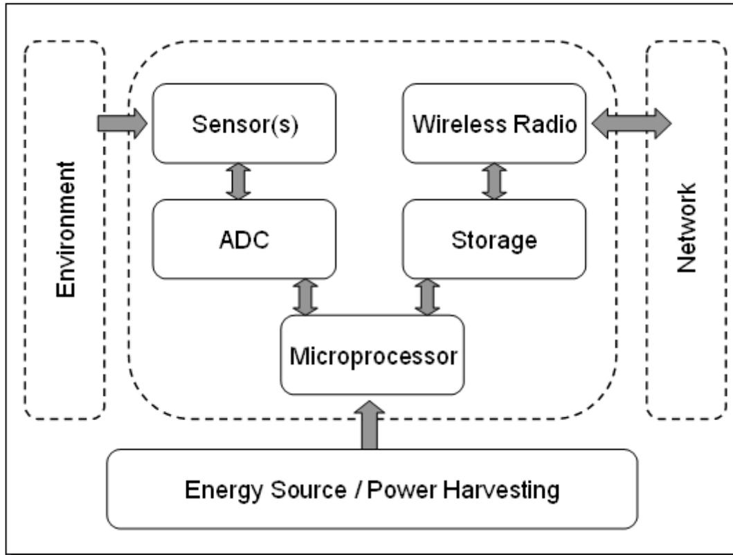
**Figure 2.2. Typical architecture of a wireless sensor node [11]**
