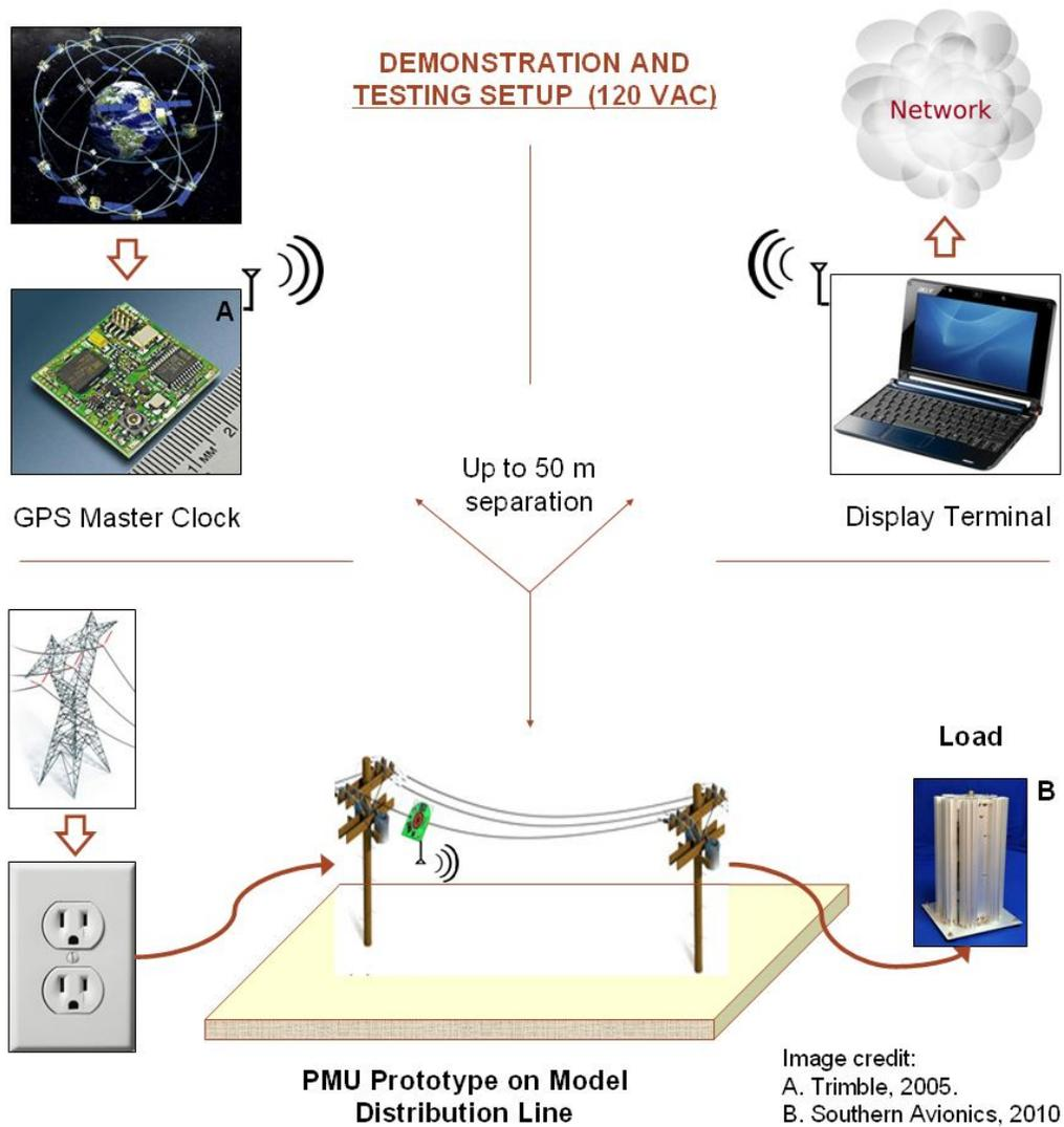
**Figure 4.2. Author's test setup for concept next generation PMU**
