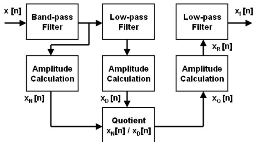
*Figure 4.9. Sezi method frequency measurement algorithm [31]*
