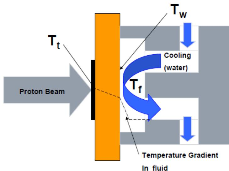
Figure 5 : Target Cooling
