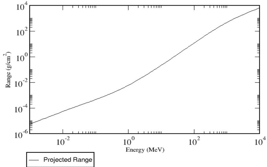
**Figure 3 : Range of Protons in Nickel**
