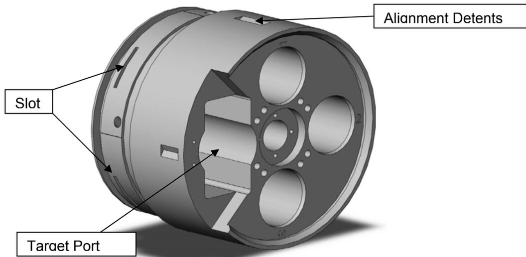
**Figure 8 : Modified Target Carousel**
