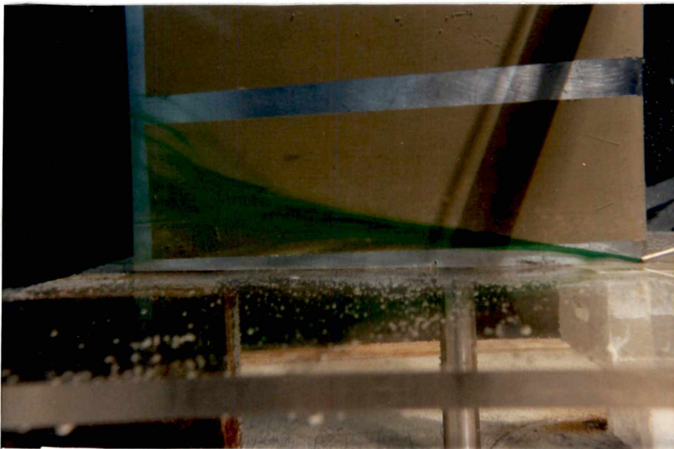
Figure 3.21 Views of the flowfield with suction applied through 4 holes Q = 21.0 cc/sec and C_Q = 0.0275 , at \beta = 6^\circ ( V_\infty = 8.91 cm/sec, Re = 16060 )
