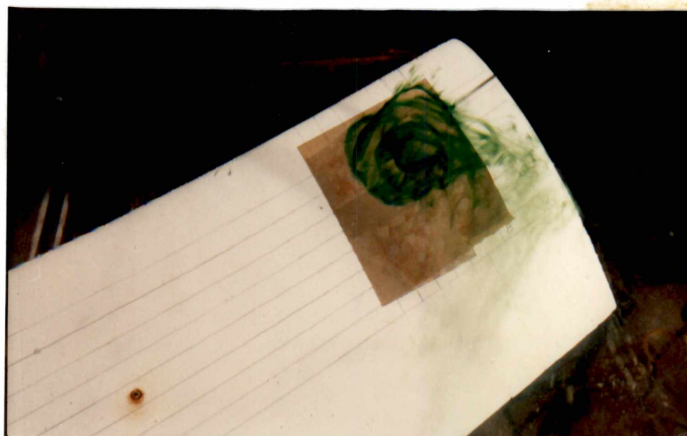
Figure 3.23 Views of flowfield with no suction applied at \alpha = 30^\circ (top picture), 40^\circ (bottom picture) ( V_\infty = 8.91 cm/sec, Re = 14370 )
