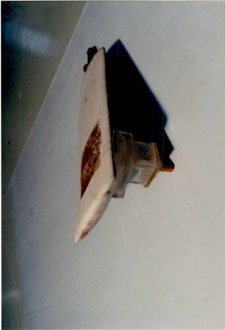
Figure 2.12 Forward-swept wing set - up, NACA 0012-64
