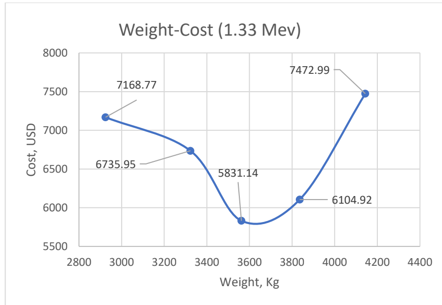
Figure 6. Weight vs. cost for 60 Co energy at 1.33 MeV.
