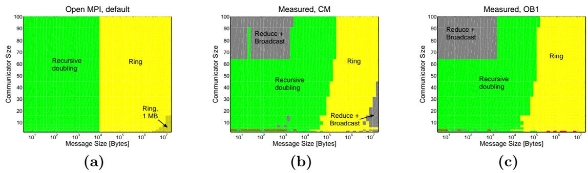
Figure 6.24: Allreduce decision maps on Cray XT4 (a) default Open MPI, and measured using (b) CM PML (c) OB1 PML.
