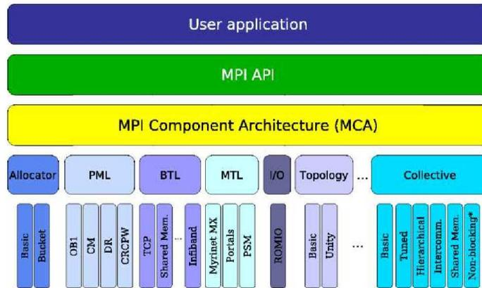
Figure 3.1: Modular Component Architecture in Open MPI.
