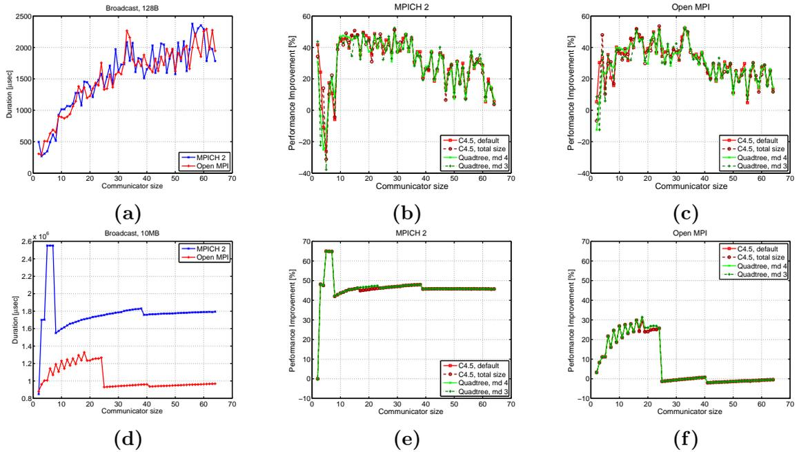
Figure 6.23: Performance improvement over native (b), (e) MPICH 2 and (c), (f) Open MPI Broadcast using (a), (b), (c) 128 B and (d), (e), (f) 10 MB message sizes.
