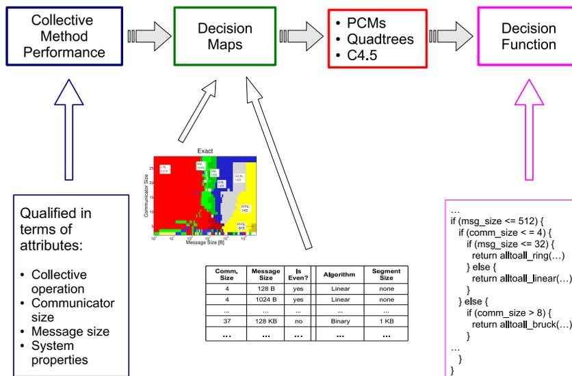
Figure 1.1: Platform-specific tuning process.
