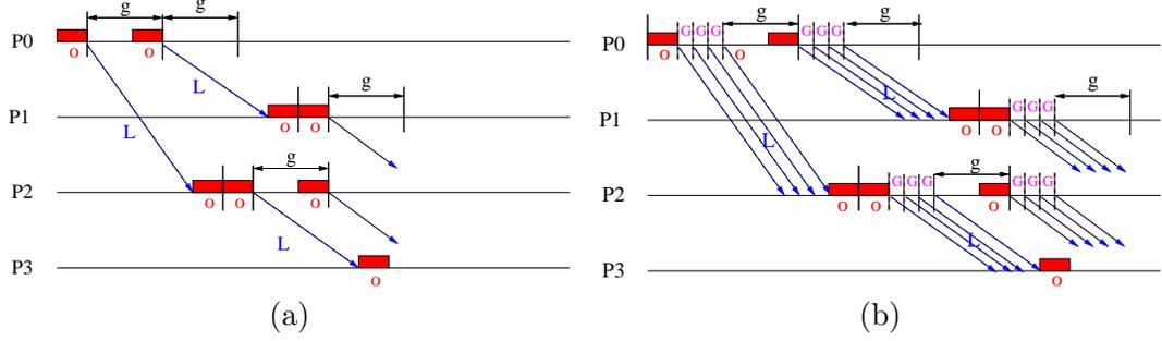
Figure 4.14: (a) LogP and (b) LogGP model parameters. The figure shows broadcast-like communication pattern:  $P0 \rightarrow \{P2, P1\}$ ,  $P1 \rightarrow \{\dots\}$ , and  $P2 \rightarrow \{P3, \dots\}$ .
