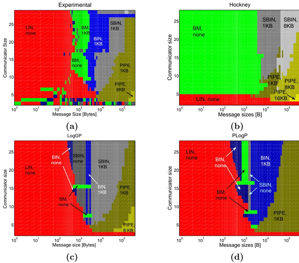
Figure 6.3: The best broadcast decision map according to (a) experiment, (b) Hockney, (c) LogGP, and (d) PLogP models.
