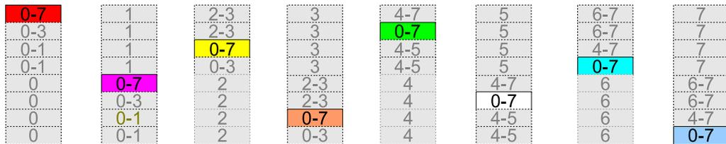
Figure 4.8: Computation phase on eight processes for Rabenseifner's original reduction algorithm. Shaded areas in data buffers are not exchanged.
