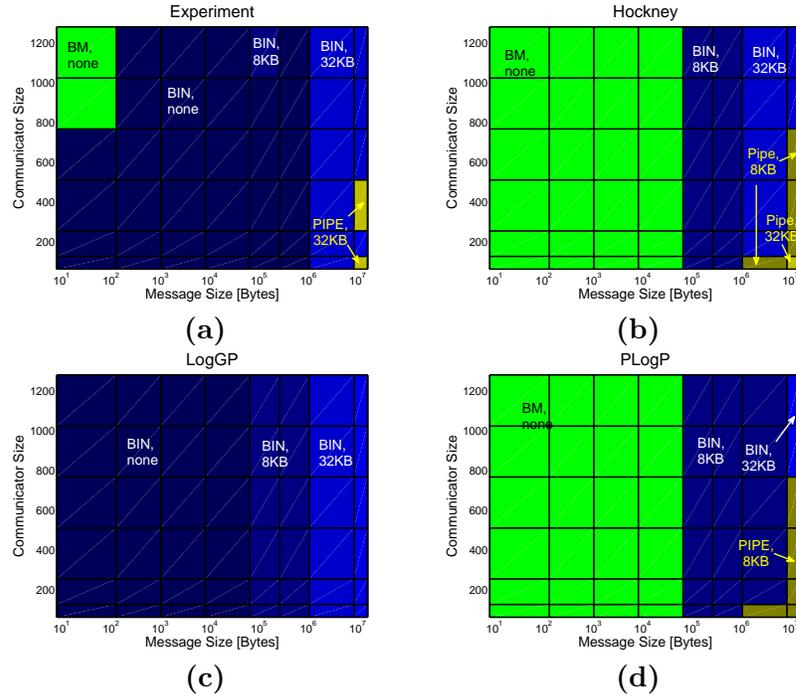
Figure 6.20: Reduce decision maps for Thunderbird system: (a) measured, and (b) Hockney, (c) LogGP, and (d) PLogP model based.
