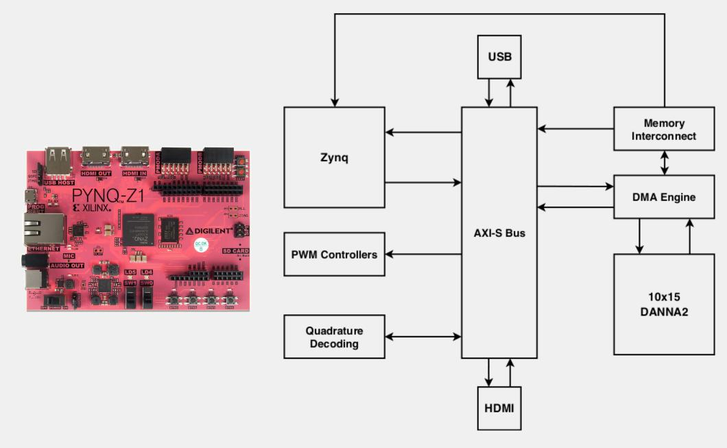
The robot communicates with its peripherals via AXI4-Stream. The sensors are connected through USB and the encoders are directly connected to hardware quadrature decoding blocks on the FPGA. Similarly, the motor controllers are connected to hardware PWM controllers on the FPGA.
