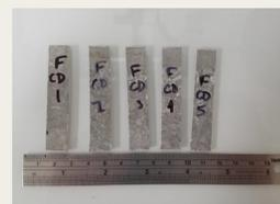
Once the plate is fabricated (Figure 3: Left), along (with reference to conveyor side) side is marked. Samples are taken from the plates according to ASTM standards (Figure 3: Right).
