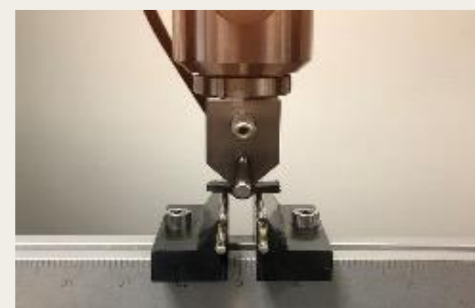
Figure 5: Test Resources 3-point Bending Test Set-up for Flexure and ILSS Test.
