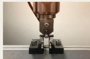
tests using ASTM standards D790 and D2344 respectively in Test resources frame located at FCMF, UTK.
