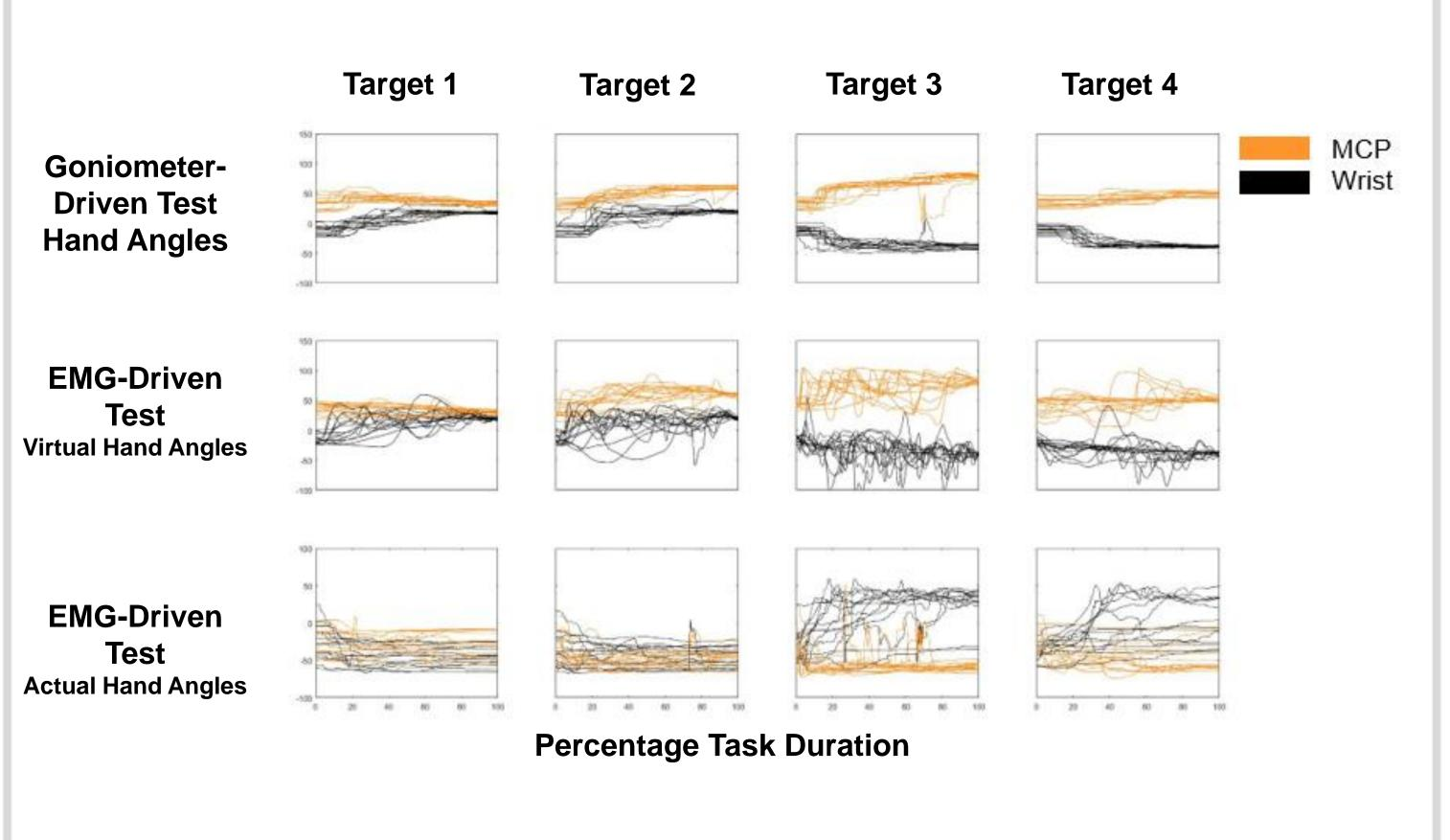
There was a trend of better overall task performance for the goniometer-driven test (G) than for the EMG-driven test (EMG).
