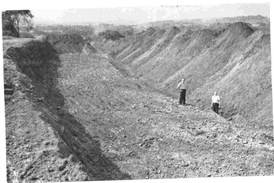
Figure 1. The soil overburden, the phosphate and the removed overburden in the phosphate mining operation.
