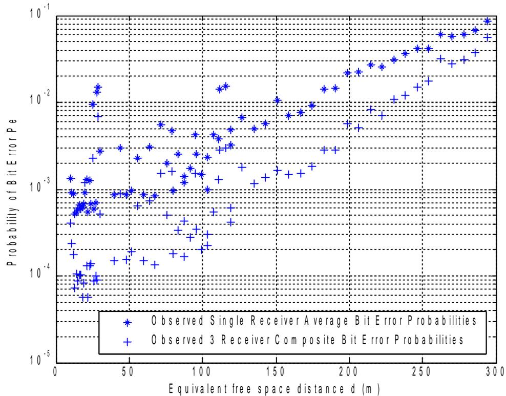
Fig 14: Observed Bit Error Probabilities for 3 Receiver Composite Case and Single Receiver Average
