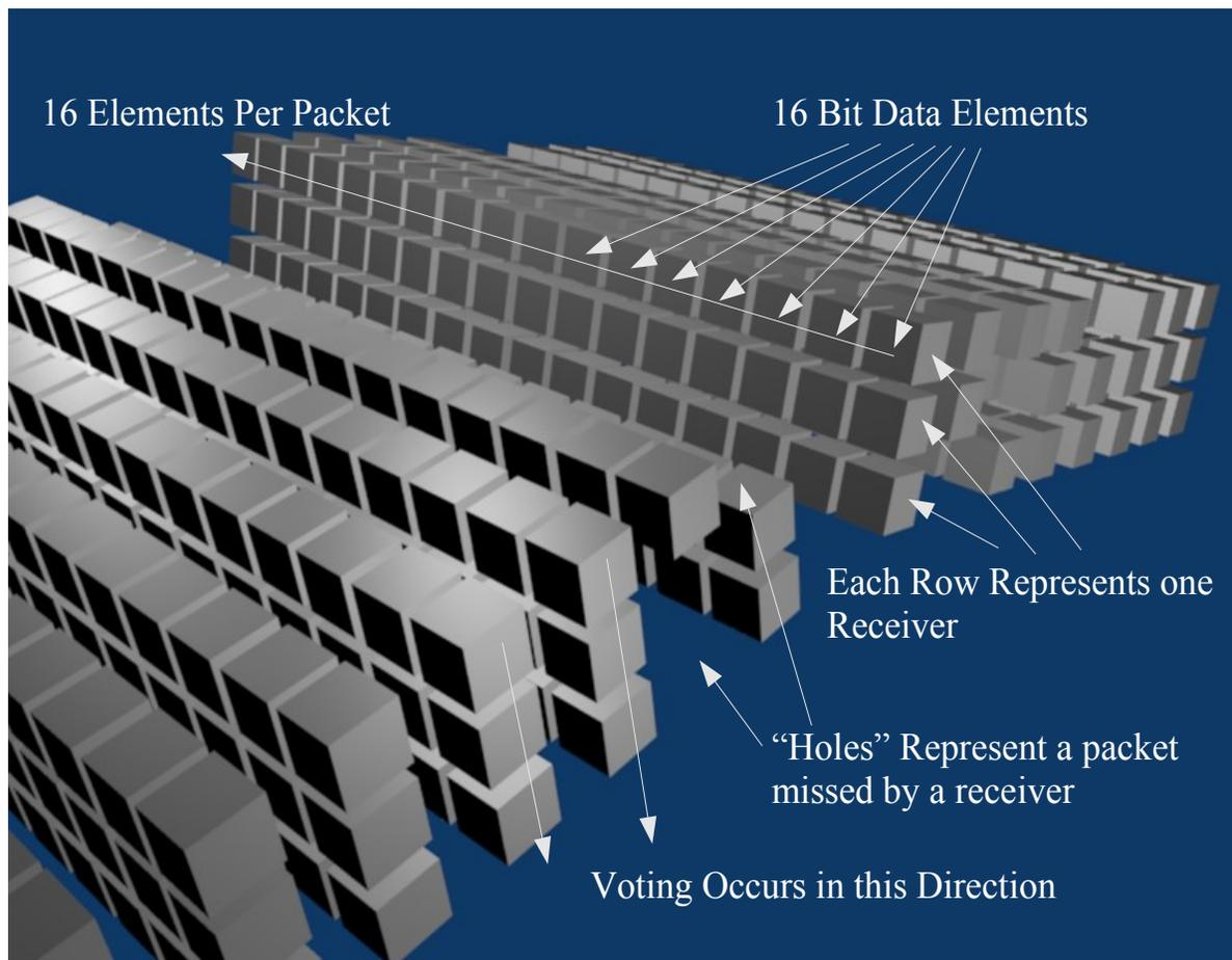
Fig 5: Structure of 3 Dimensional Packet Array
