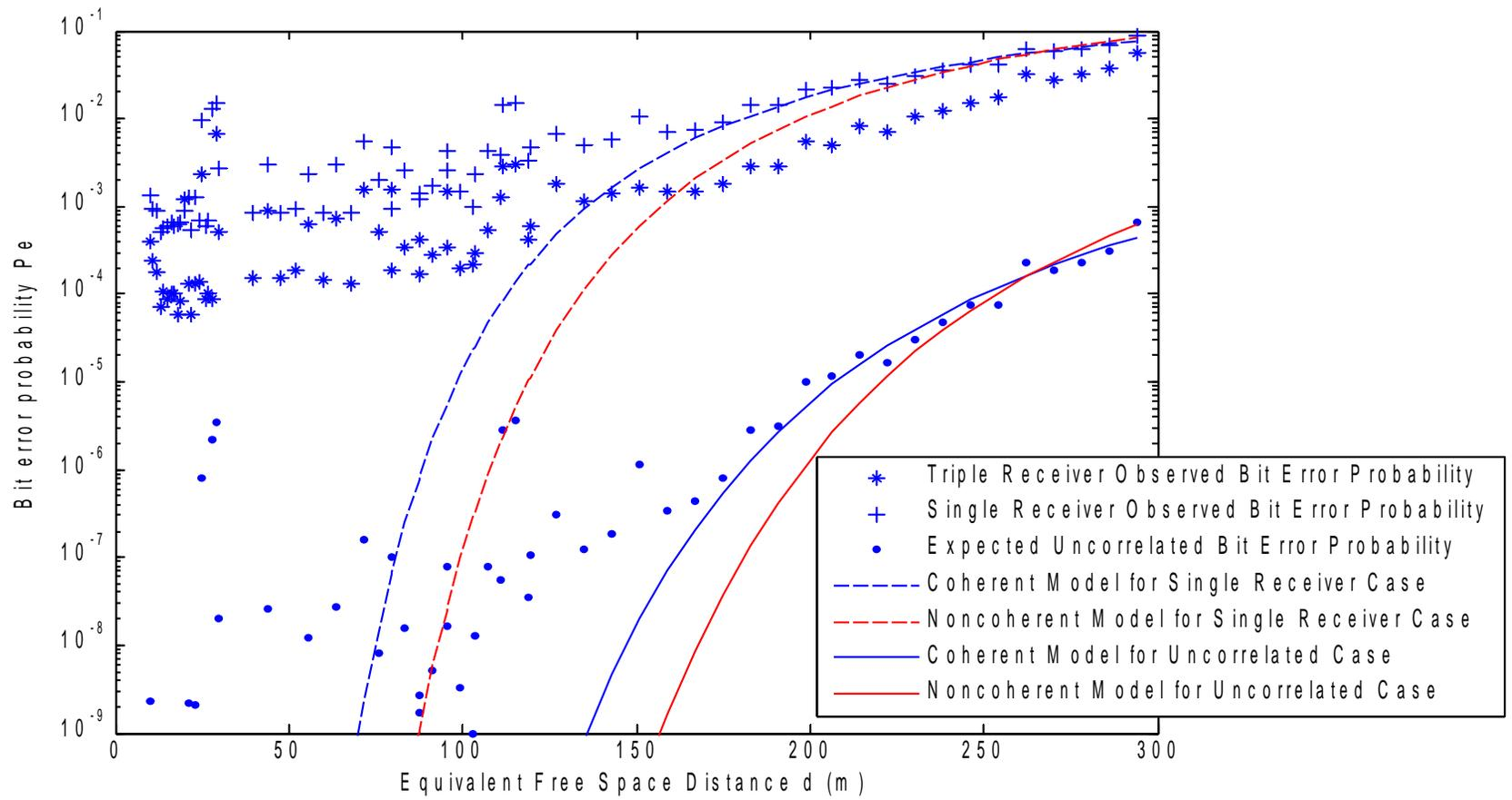
Fig 15: Triple Receiver Bit Error Probability Envelope
