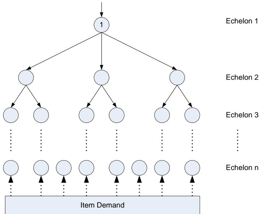
Figure 4.2: The arborescent structure of the distribution network
