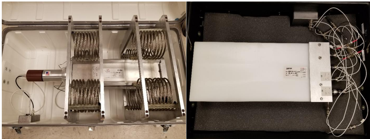
Figure 2. Photos of Ortec NAI-SS-4-P system in their ruggedized cases including the 4"-by-4"-by-16" NaI scintillation detector (left) and the four 3 He tubes in polyethylene moderator (right)
