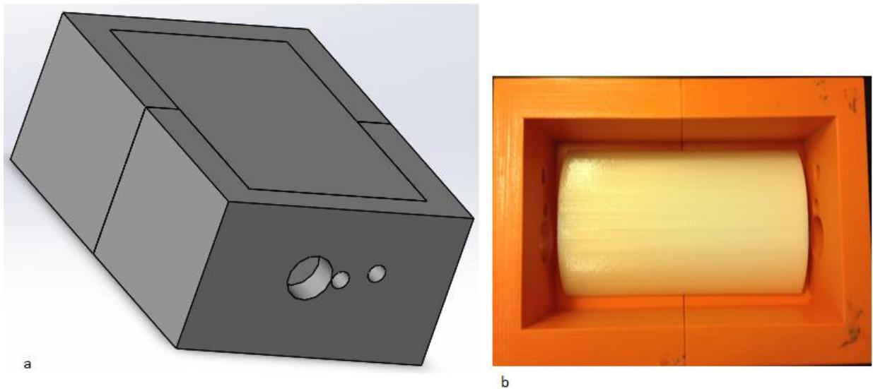
**Figure 4:** (a) The lung piece, represented by the rectangle on the top of the 3D model, fits perfectly in the mold with no room on the sides. (b) The revised lung piece fits inside of the mold with plenty of room on the sides for the Ecoflex material to flow by and also leave the skin layer undamaged.
