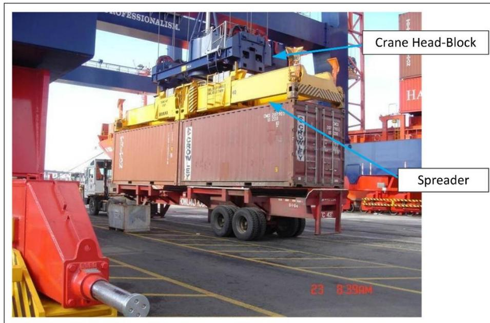
Figure 1. Container Crane Spreader
