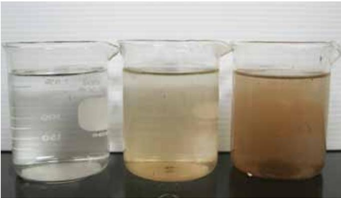
*Figure 2. Varying turbidity levels in water (from left to right: 0, 200 and 1,500 NTUs).*
