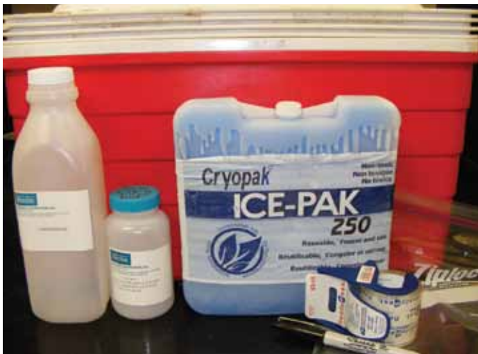
Figure 1. Water sampling supplies: cooler, ice or ice packs, sampling bottles, marker, zip-close bag and tape.
