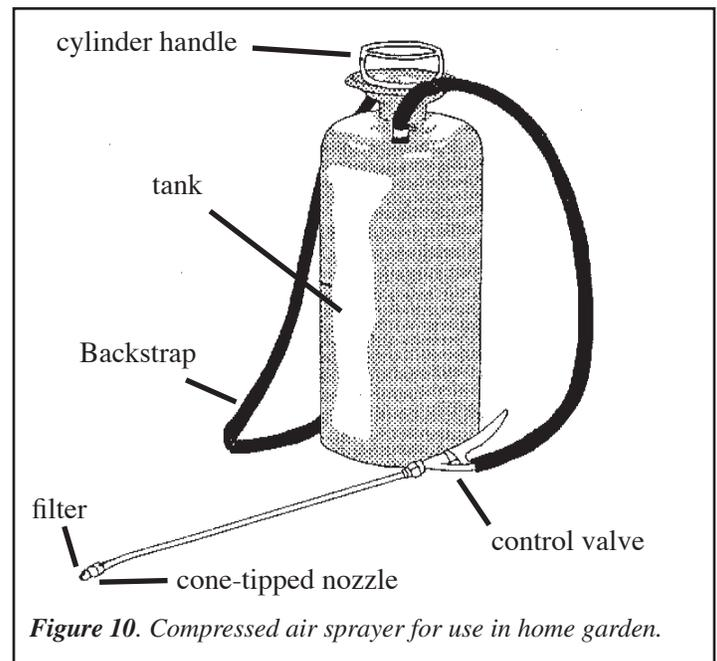
**Figure 10.** Compressed air sprayer for use in home garden.
