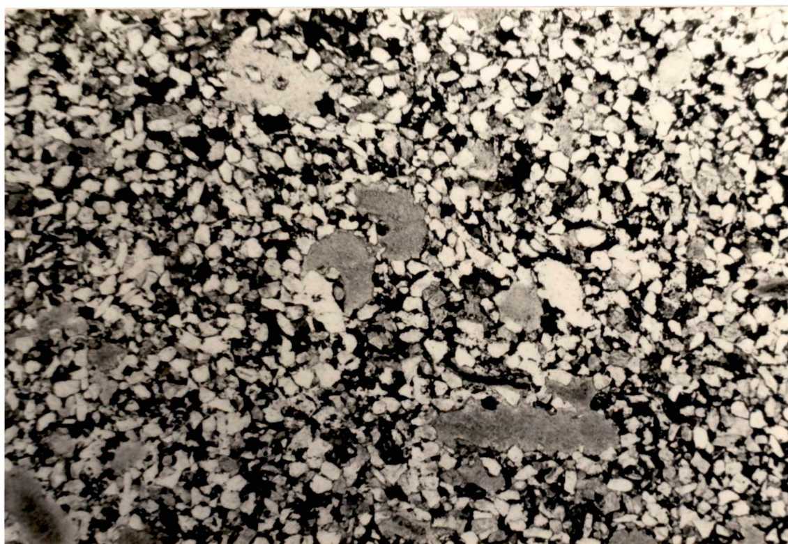
Figure 19. Typical Lithology of Facies AH Composed of Quartz Grains, Hematite Replaced and Unreplaced Bioclasts, Hematite Cement, and Calcite Cement. Field of View from Left to Right is 2mm.
