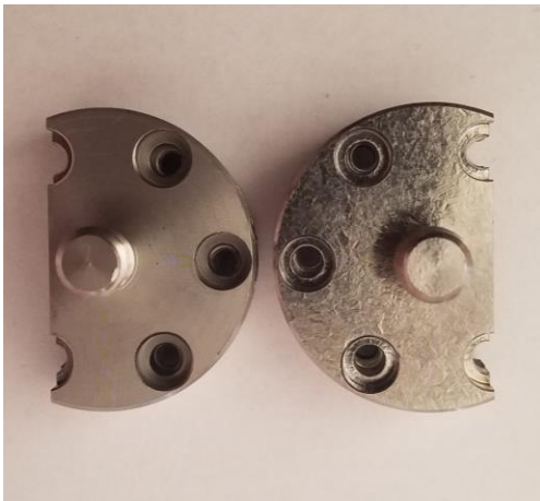
Fig. 3 Comparison of Ti-64 lids from sample canisters used in high-temperature experiments at the SNS
