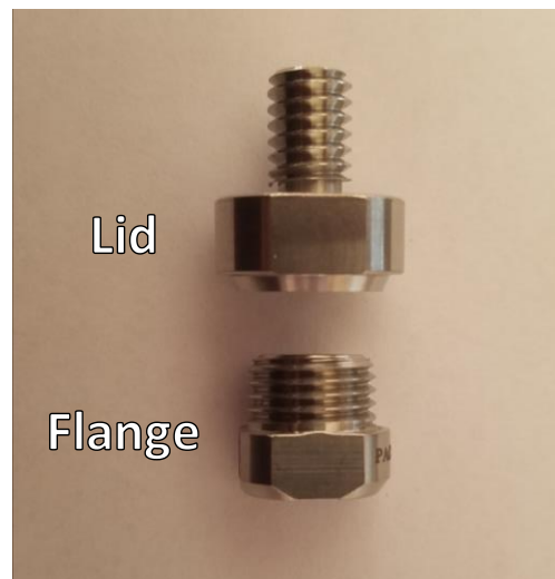
Fig. 12 Canister lid and flange assembly, provided by ORNL, using screw threads to join the Ti-64 lid and flange rather than Mo screws.
