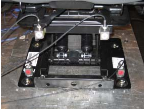
Figure 4.5a: Seat test stepup:Accelerometer instrumentation front view
