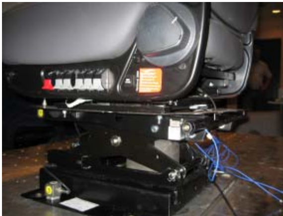
Figure 4.5b: Seat test stepup:Accelerometer instrumentation left view
