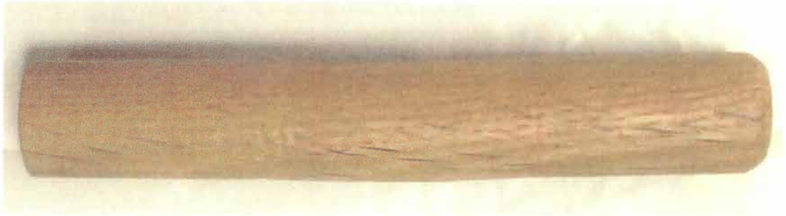
Figure 3.5: Vertical marks on peg show signs of crushing failure
