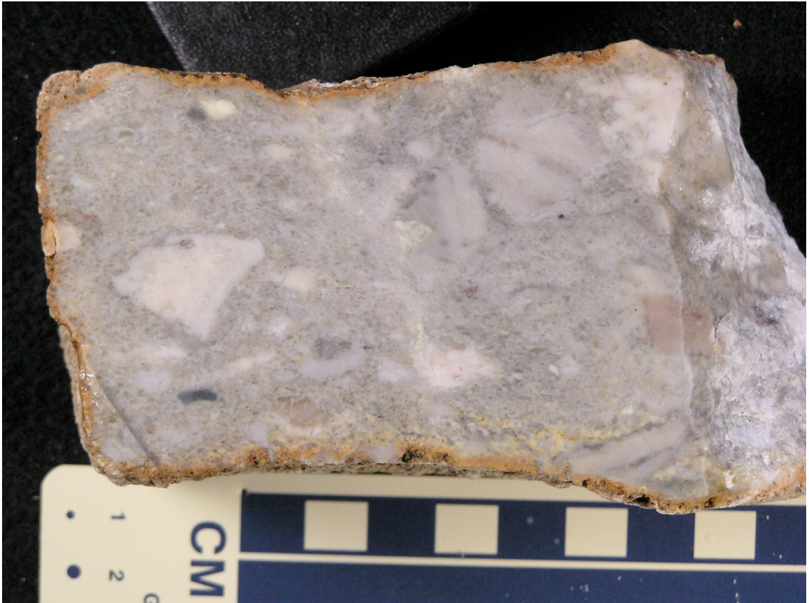
Figure 13: Cut surface of sample from Lostkey breccia. Clast composition is dolomitic sandstone and siltstone. Matrix is authigenic quartz and feldspar and coarse-grained carbonate.
