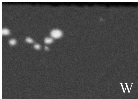
Figure 16: EPMA element maps of a 230-alloy specimen isothermally oxidized at 700°C – (a) Backscattered Image, (b) Ni, (c) Cr, (d) O, and (e) W.
