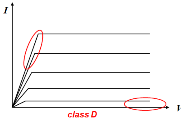
Figure 4.1 Operation region of class D PA
