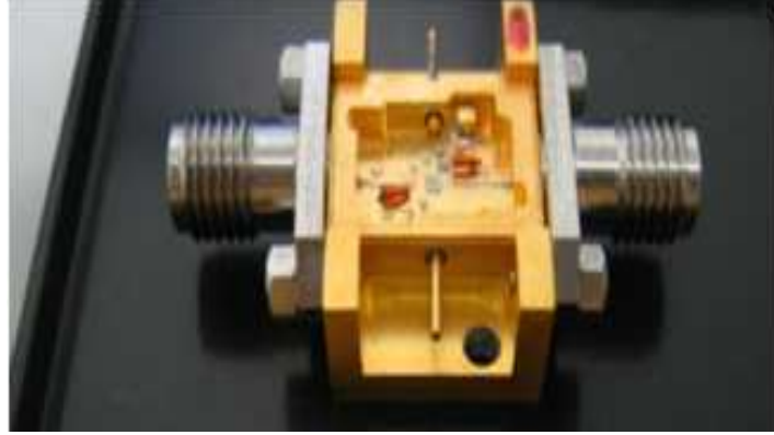
Figure 2.19 Fabricated feedback PA with housing
