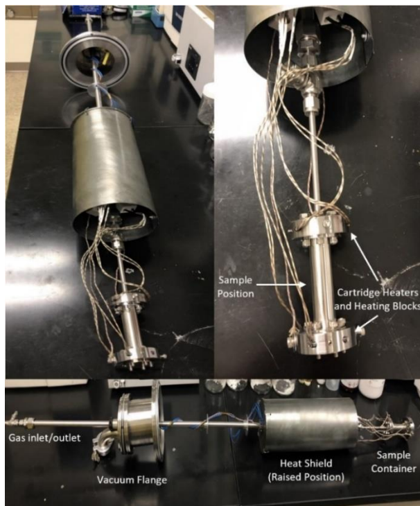
Figure 5: Custom stick furnace for VISION experiments. The vanadium heat shield is in the raised position, which is lowered for during measurements.
