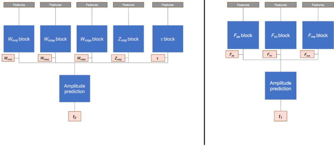
Figure 4.3: Architecture of DDCCNet_v3, where a) shows the architecture of the t_2 prediction head and b) shows the architecture of the t_1 prediction head.
