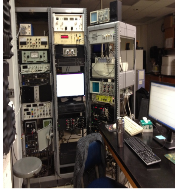
Figure 3. The Kopf model 650 micropositioner advanced the microelectrode through the brain. AD Instruments hardware and LabChart software were used to produce a visual representation of the neuron's membrane potential.
