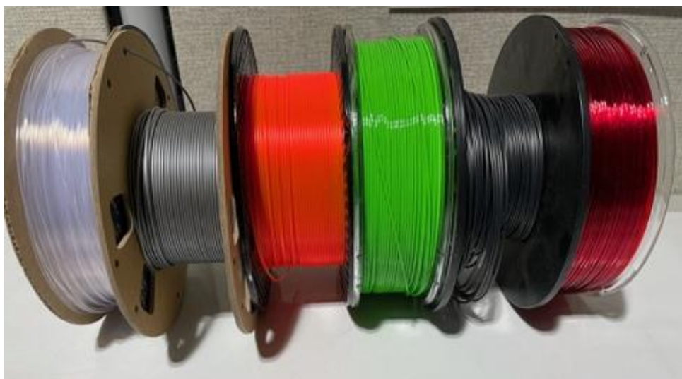
Figure 3.2. Filament spools. From left to right: PLA, PETG, PVB, NGEN, ABS, CPE.
