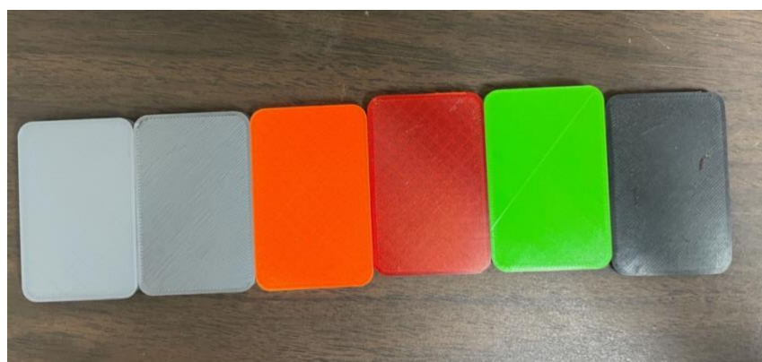
Figure 3.5. Surface quality samples. From left to right: PLA, PETG, PVB, CPE, NGEN, ABS.
