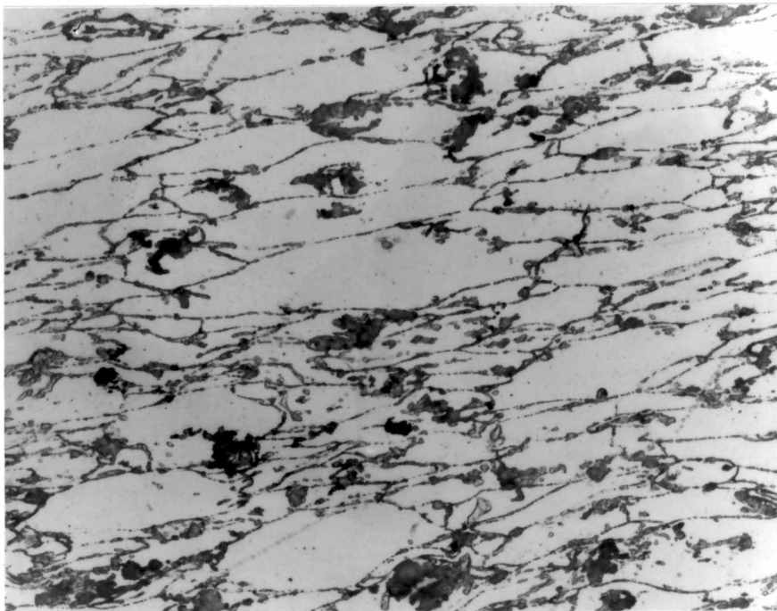
B) Tensile, Al-123, #3-6, 400X (bulk)
