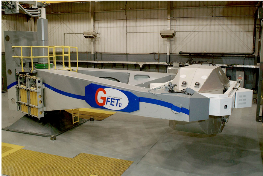
Figure 3. Photograph of ATFS 400 Centrifuge Manufactured by ETC
